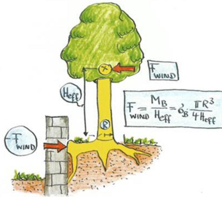
Fig 6 – Roots are likely braced against the face of the wall given the proximity of trees (above left) with some roots also likely extending below the wall (above right). Where TG1 is retained the wall also remains.
