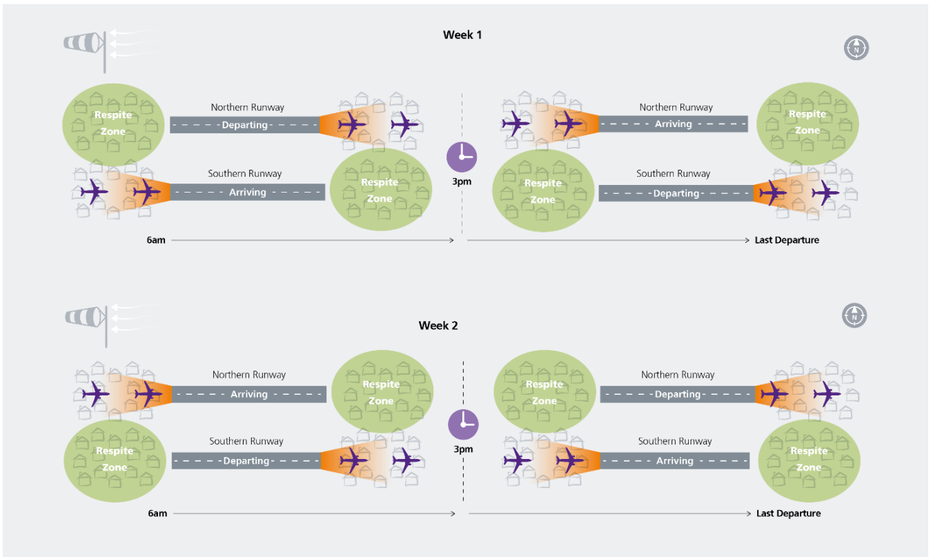
Graphic 2.4 Direction of arrivals and departures on 09R and 09L during easterly operations (proposed)
