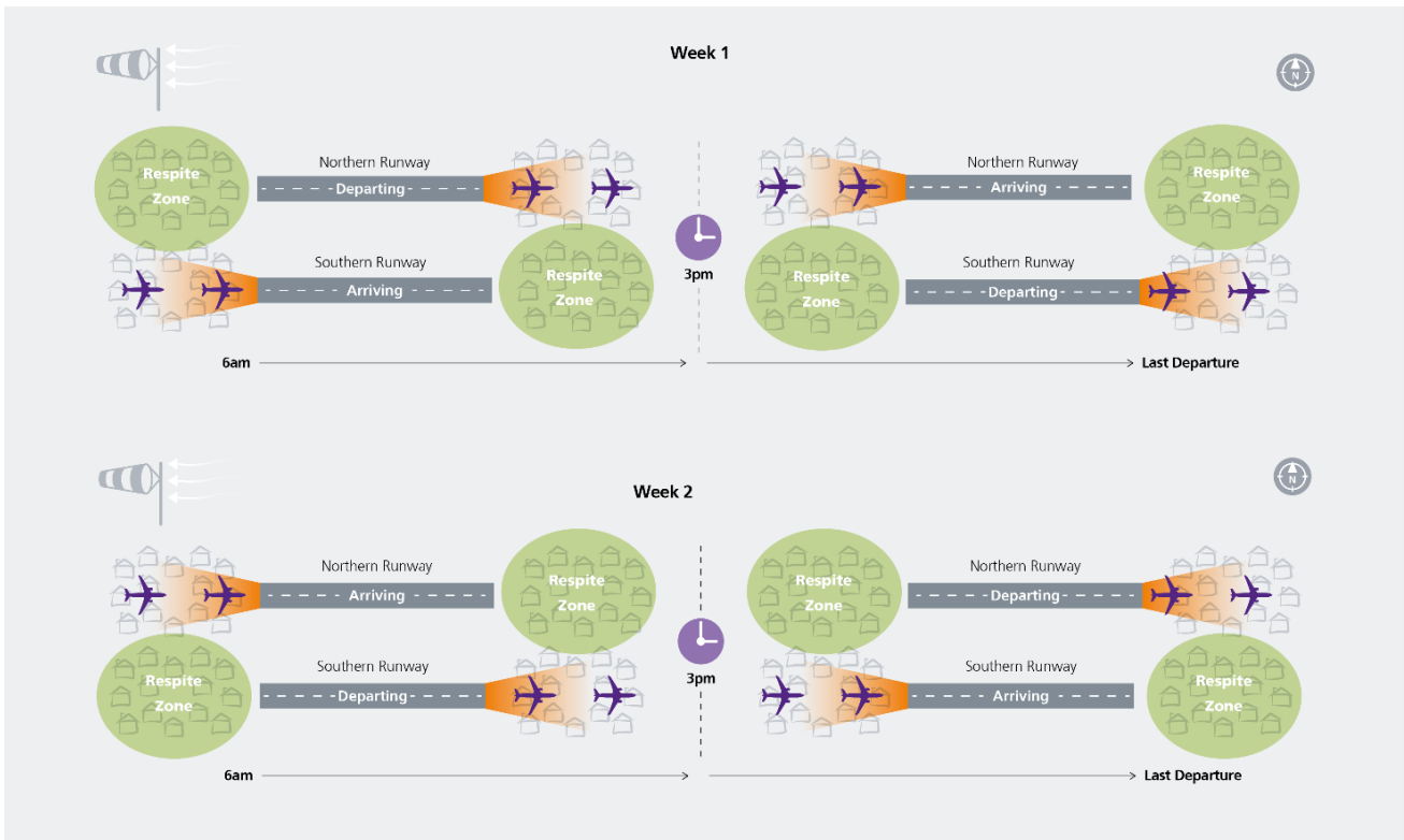
Graphic 2.5 Direction of arrivals and departures on 09R and 09L during easterly operations (proposed)
