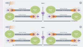
The figure above is how we would alternate the runway when on Easterly operations.
