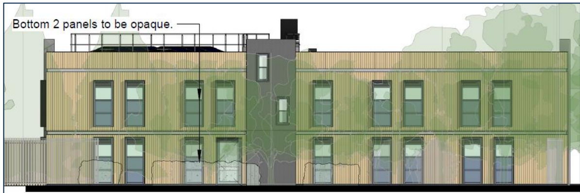
Figure 10 - Drawing showing the window design, which includes obscure glazed panels.
