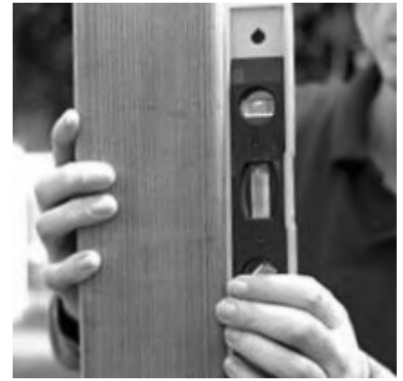
Substitute the wooden post with the upright of a ramped rail – if level, you know you have a 1:12 gradient
