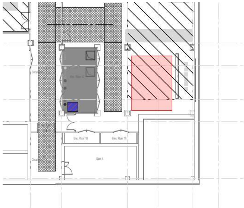
Figure 5 Space allocation for plate heat exchangers (shown in red) and risers (shown in blue) for district heating connection in the hospital building level 7 floor layout
