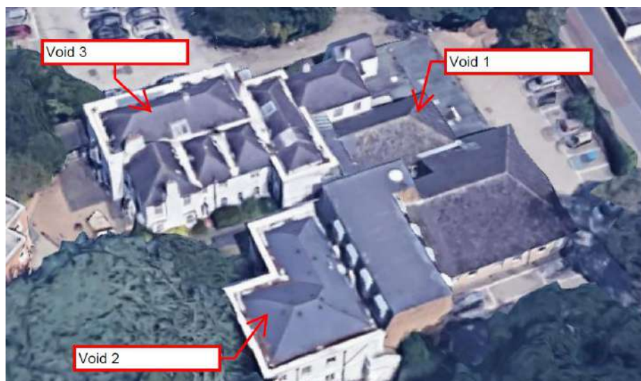
Plate 1. Location of roof voids in Building 10 (the Furze) from Google aerial image
