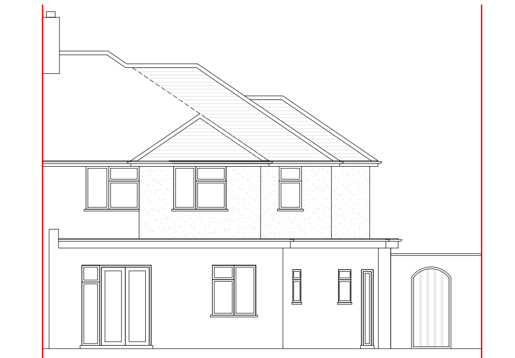
Proposed Rear Elevation Scale:1:100
