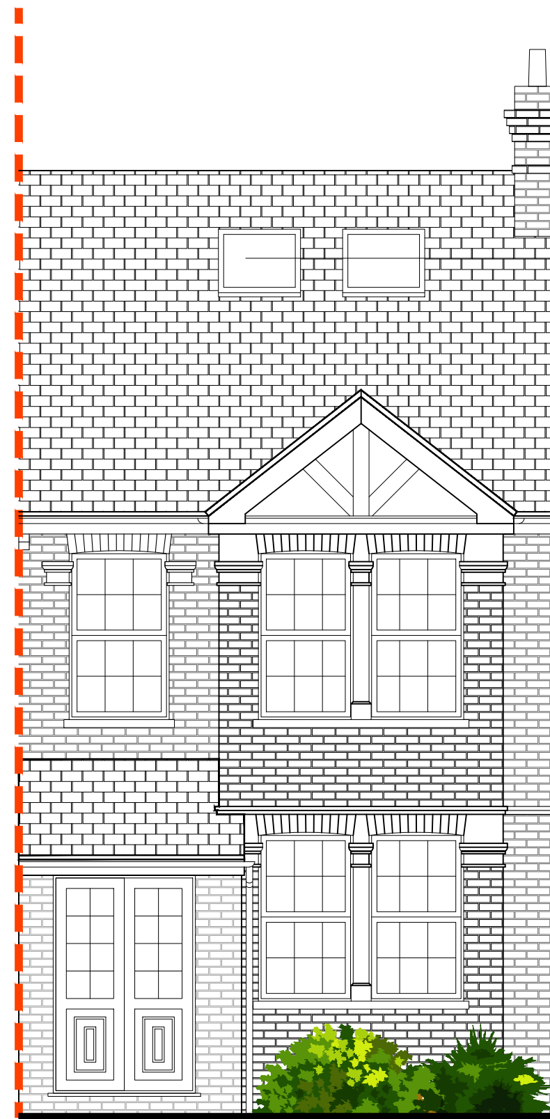
2no Velux roof light 780x980 (Client to confirm). Contractor to ensure roof light is installed in accordance with manufacturers requirements. Ensure pitch of roof meets requirements prior to construction
