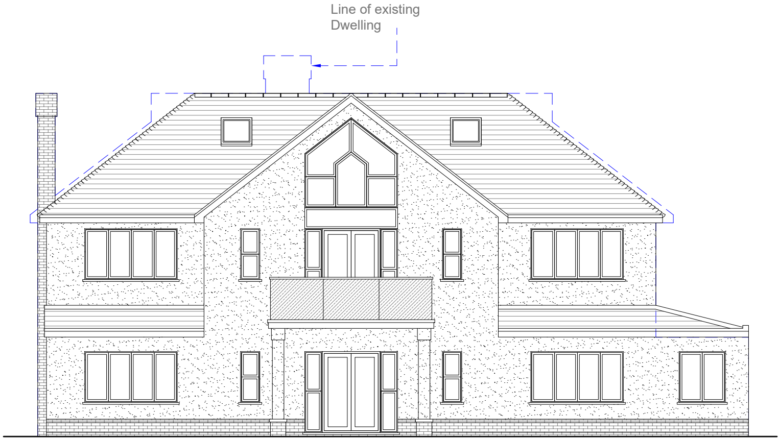
Proposed Front Elevation Scale 1:100
