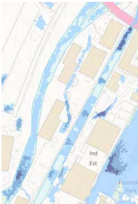
Figure 5: Flood risk from surface water
