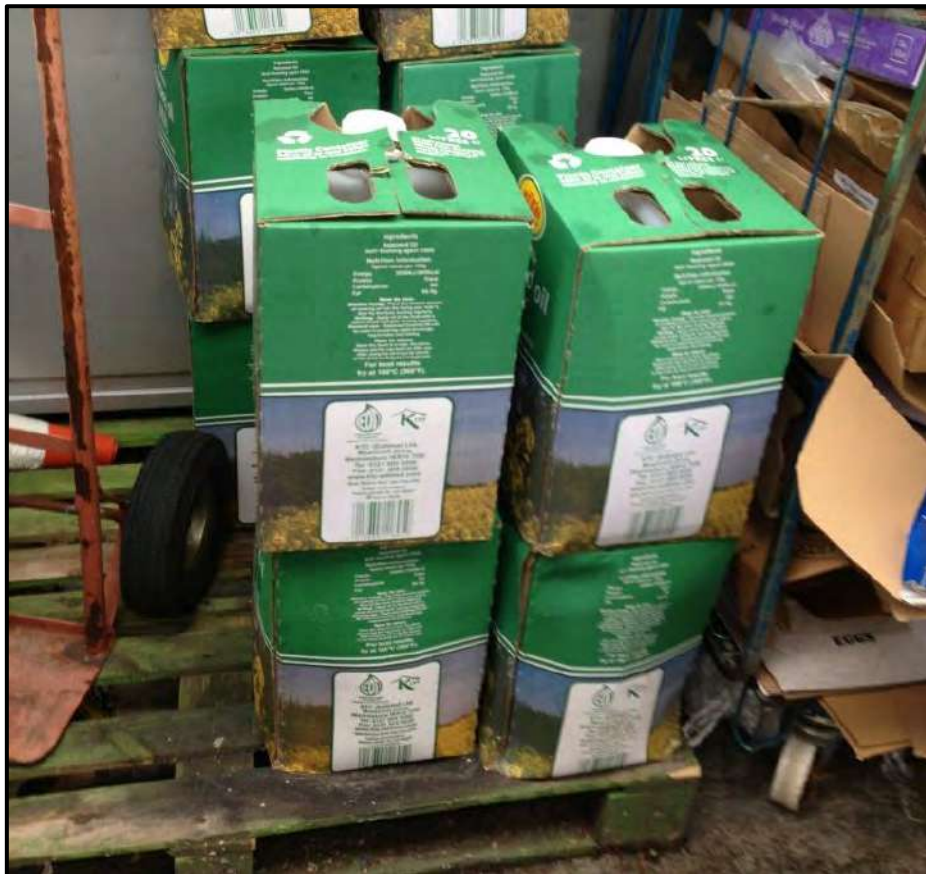
PLATE 4: WASTE VEGETABLE OIL LOCATED WITHOUT SECONDARY CONTAINMENT
