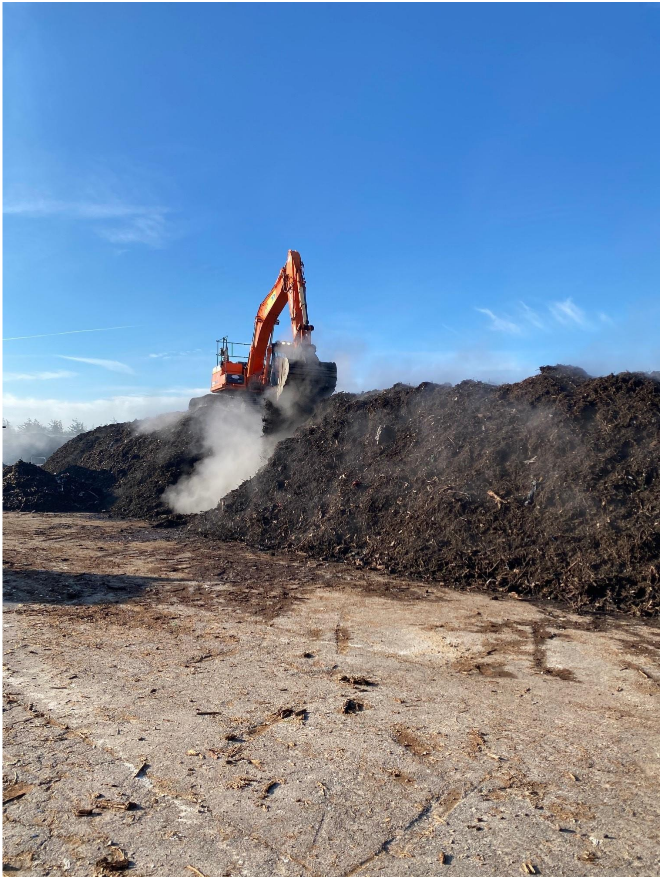
Figure 4 Turning the windrow.
