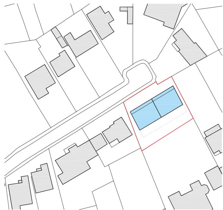
Massing Option 01 - Maximum achievable massing arranged as two dwellings positioned within the established building lines of neighbouring properties.
