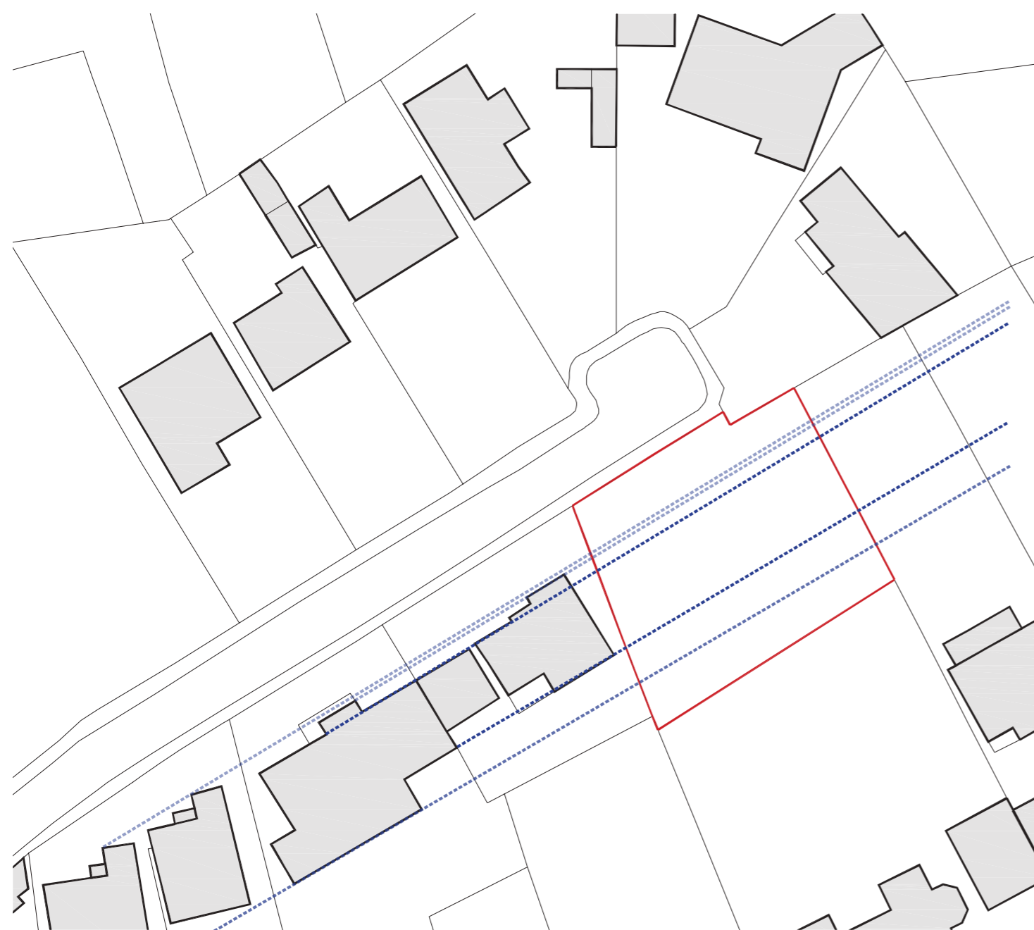
Building Line Establishment - Initial setting of building lines derived from No. 8 and No. 9 neighbouring properties to define the maximum recessed massing and establish a front building line aligned with adjacent dwellings.
