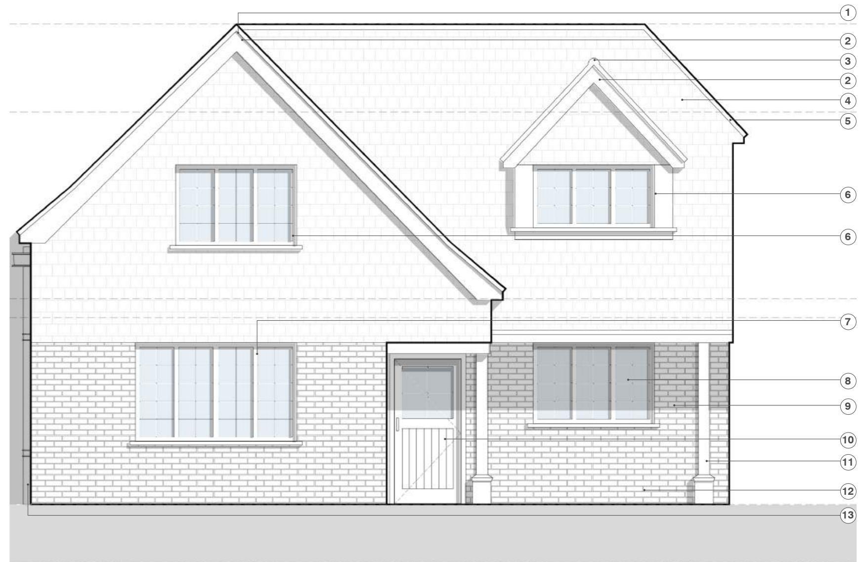
Principle Facade Study, (reflecting one dwelling but mirrored for both facades, with minor differences) Scale 1:100
