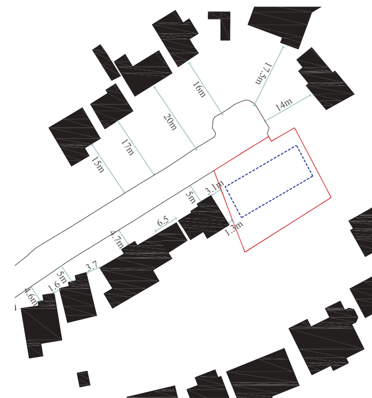
3. Establishing a perimeter area for development, from the figure ground analysis.
