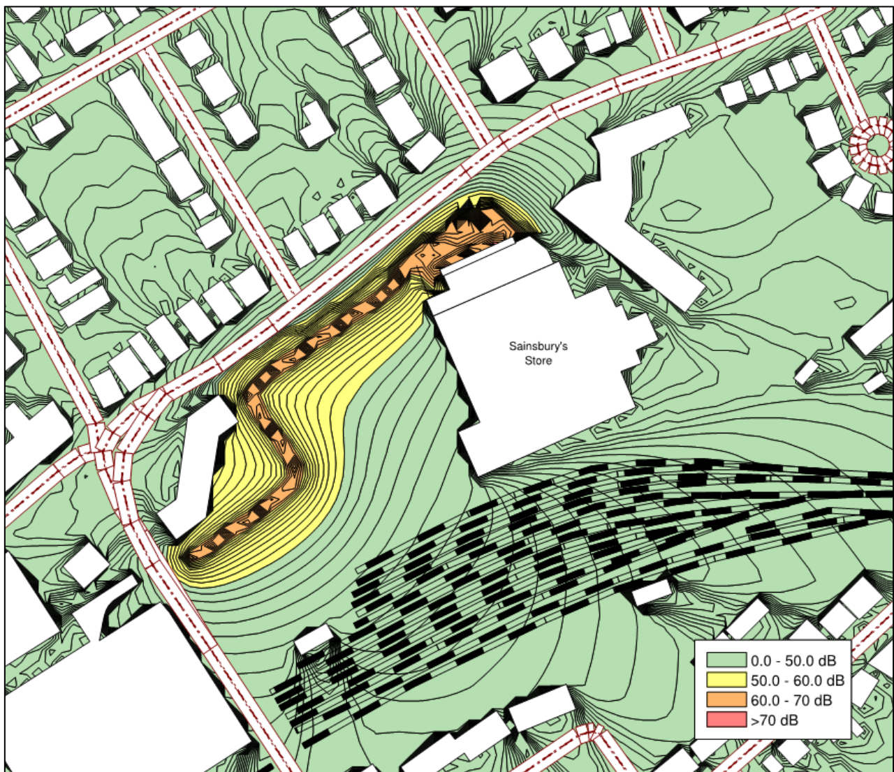
Figure 5.1 Noise Contour Plot (Daytime) L_{Aeq,1hour} – Grid Height: 1.5m
