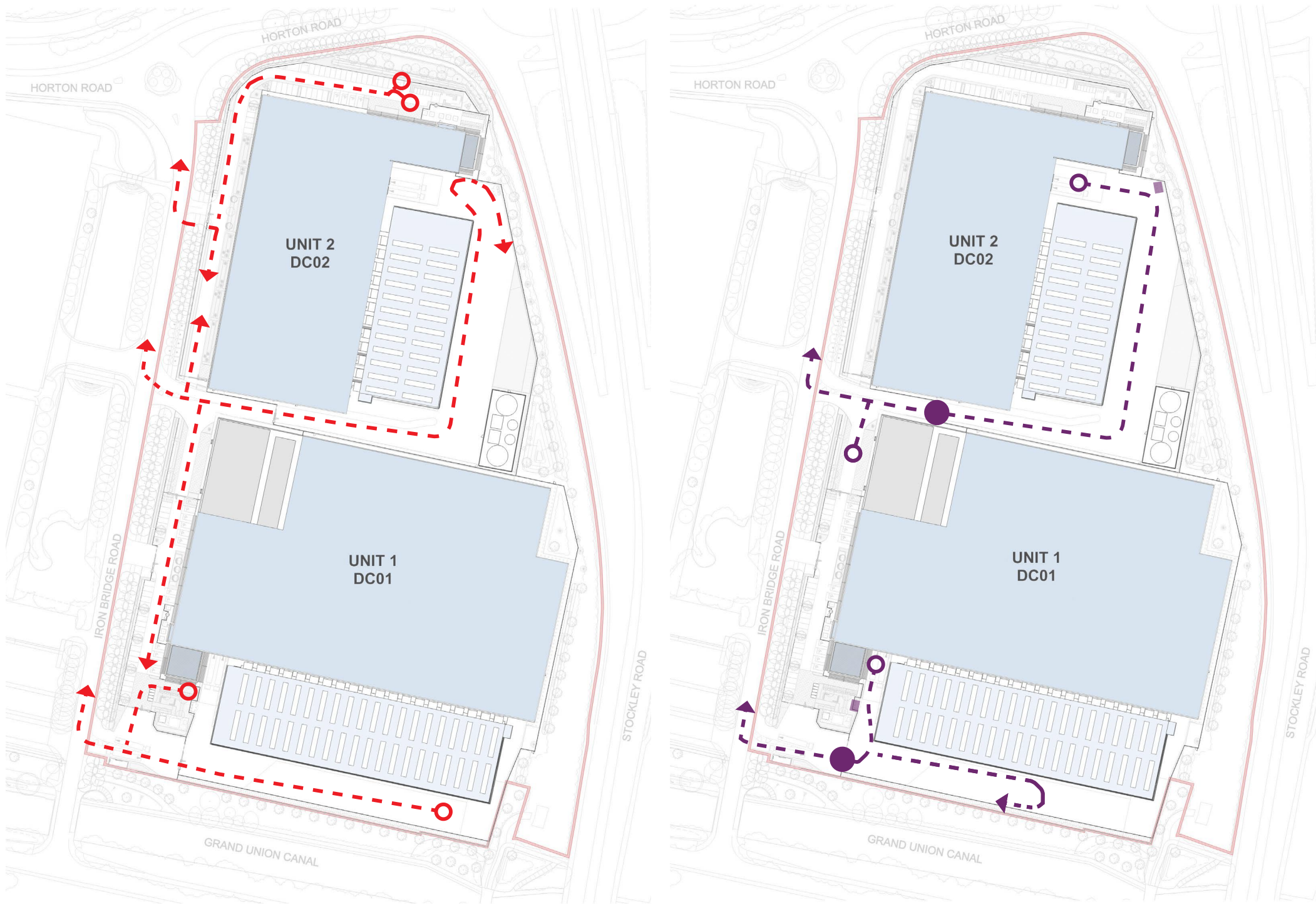
Fire Tender Access & Turning Points
