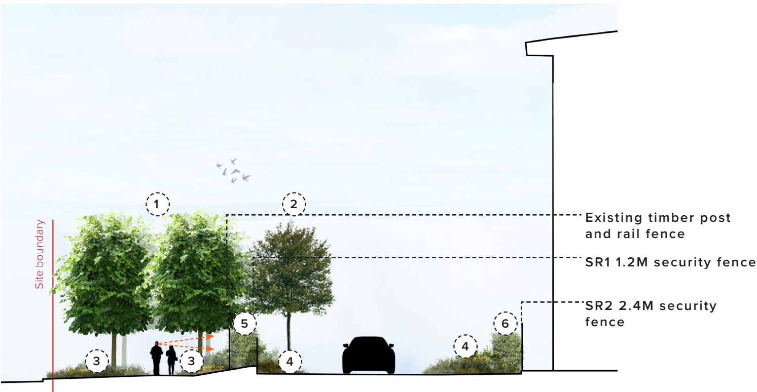
Typical section AA' along Iron Bridge Road North - Summer view
