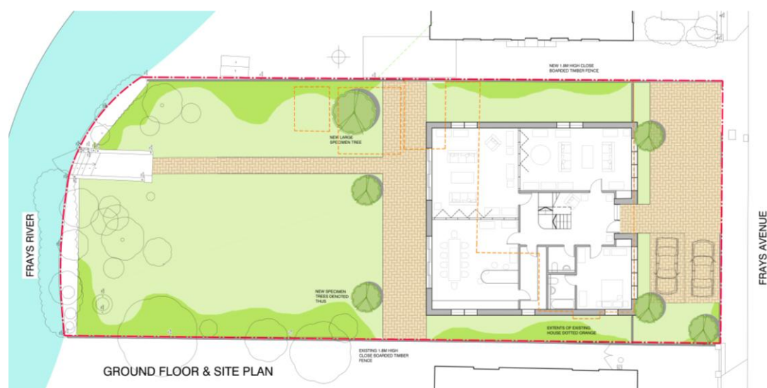
Image 1 – Extract of site layout plan showing how the position/layout of the replacement dwelling will harmonise with neighbouring properties to the north and south.
