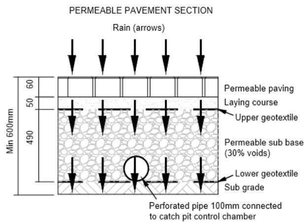
**Figure 3 Block Permeable Paving with sub-base**
