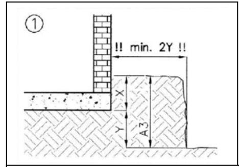
Please refer to the table on Page 2. A3 relates to the 'Excavated Overall Height' dependent on shaft and tank type
