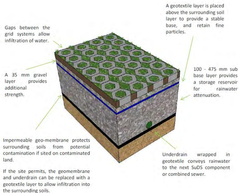
Figure 5: Plastic or Grid Permeable Paving with Sub-base
