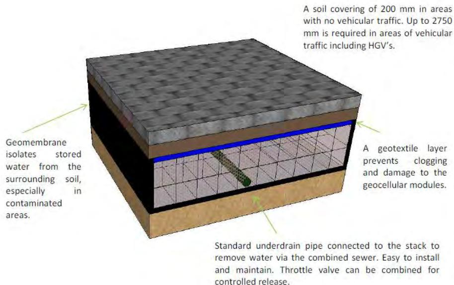
**Figure 4: Block Permeable Paving with Geocellular Module**
