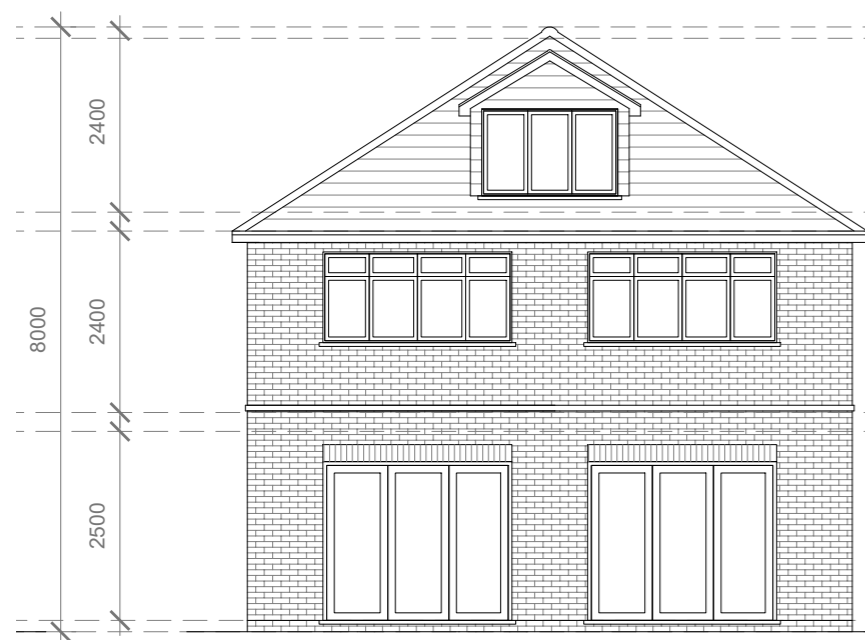
Proposed Rear Elevation Scale 1:100
