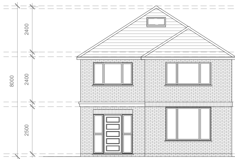
Proposed Front Elevation Scale 1:100
