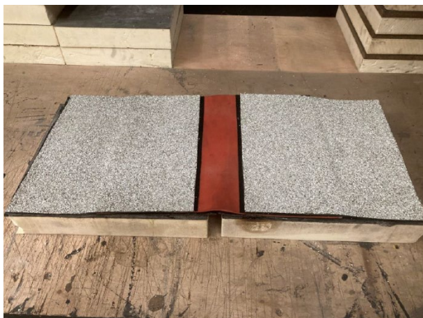
7) Ensure care is taken to avoid directly torching the joint ( temporary protection of exposed joint )
