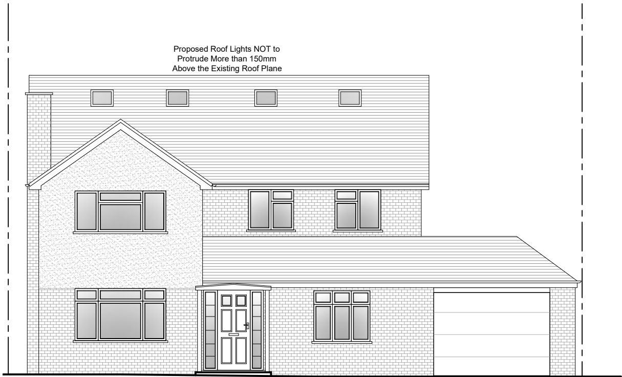
Proposed Front Elevation Scale 1:100
