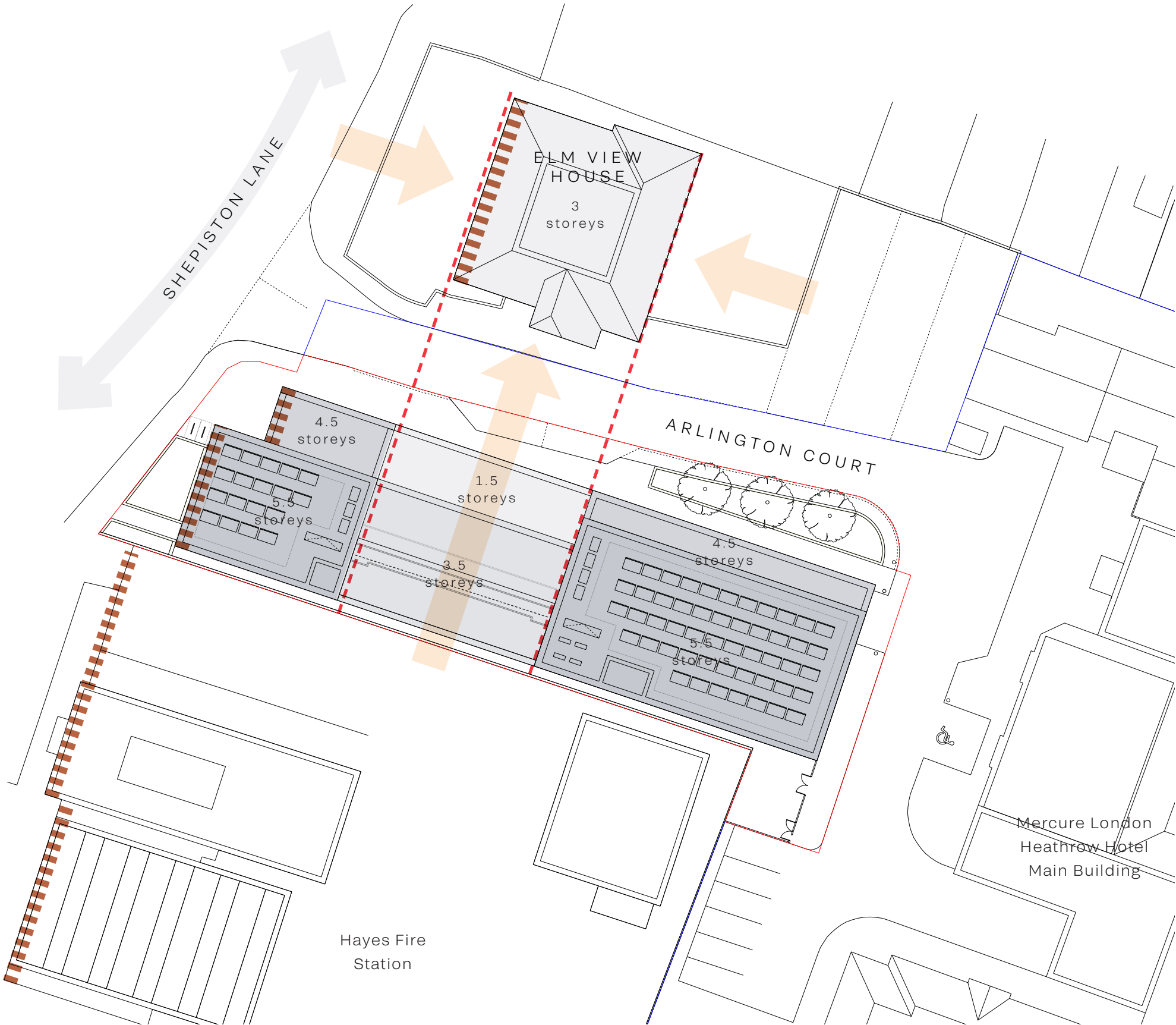
An early assessment of daylighting impact to comply with BRE guidelines
