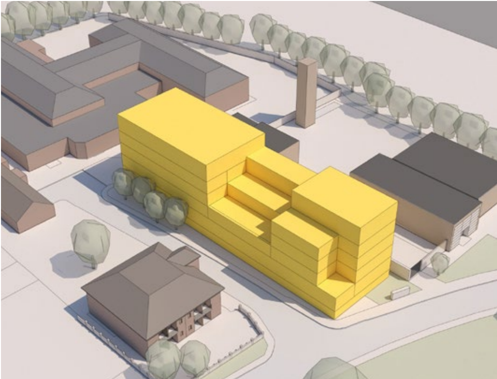
The developed volume showing a refined massing strategy complying with BRE guidelines
