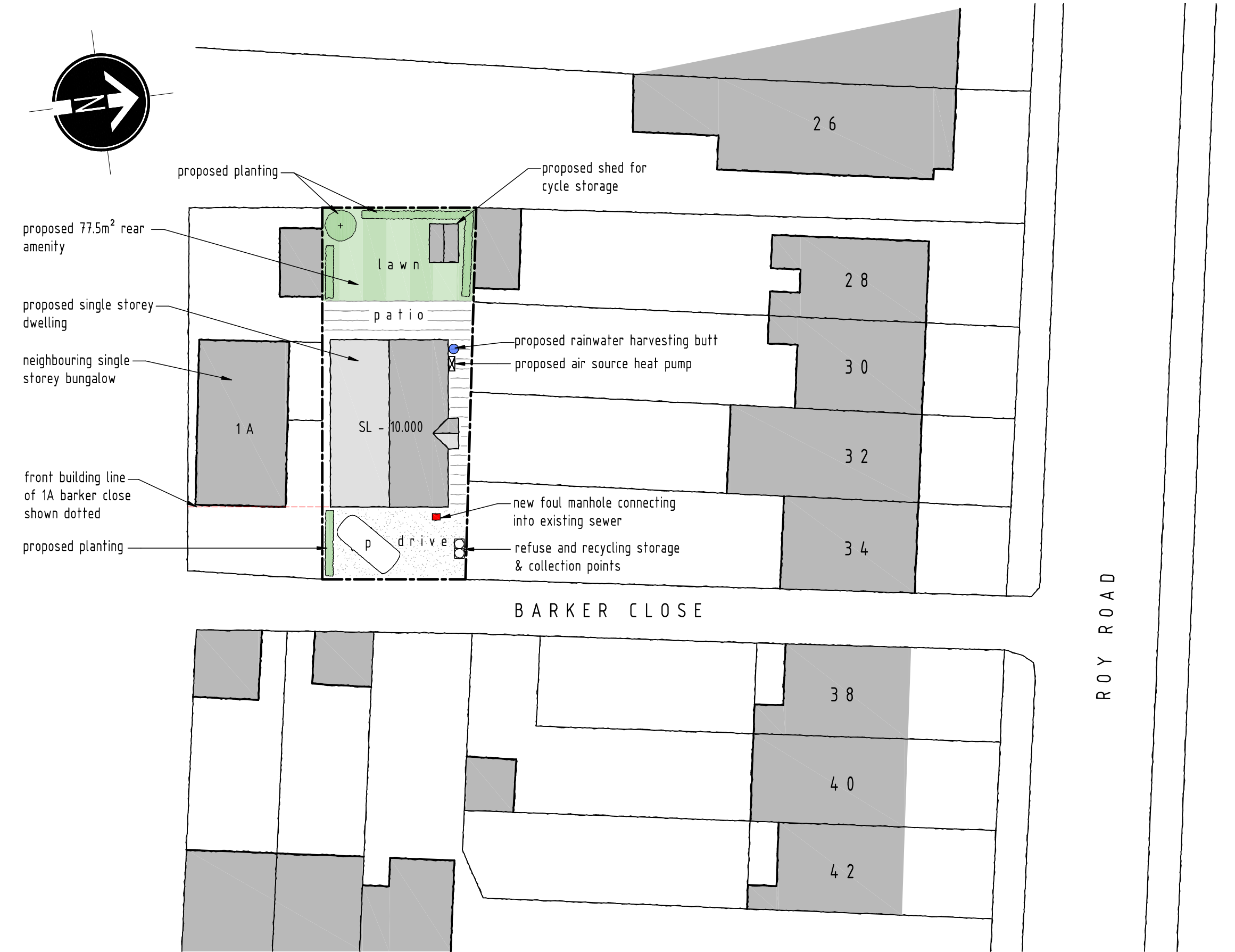
PROPOSED SITE LAYOUT PLAN SCALE 1:250
