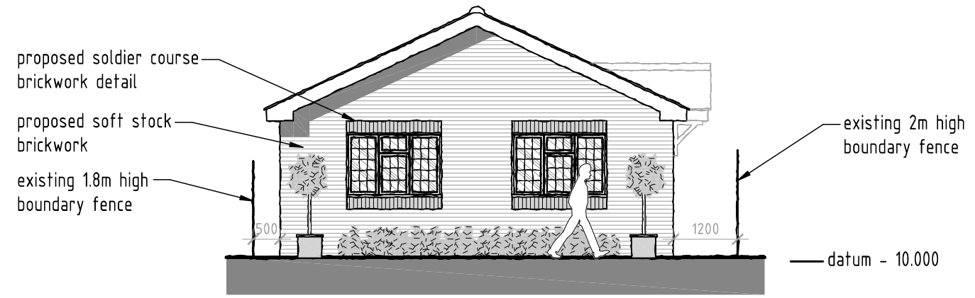
PROPOSED FRONT ELEVATION SCALE 1:100
