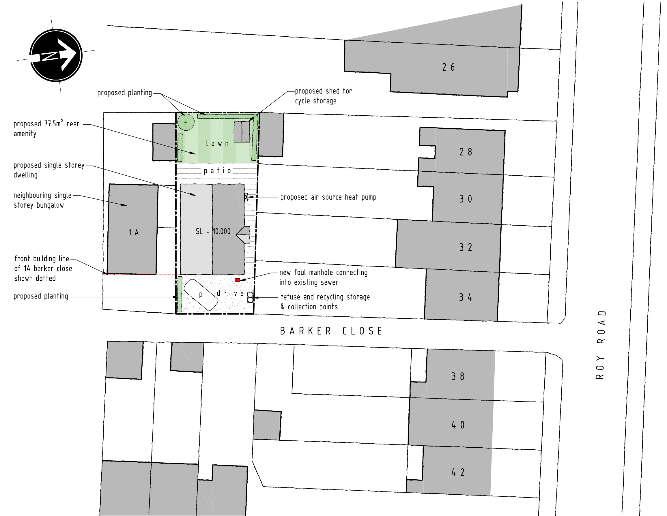
PROPOSED SITE LAYOUT PLAN SCALE 1:250
