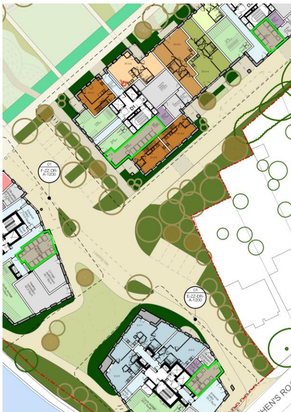
Figure 3-11 Residential Waste Store Configuration – Plots D1/D2/E/F
