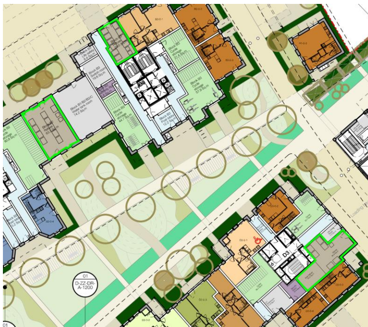
Figure 3-13 Residential Waste Store Configuration – Plot C
