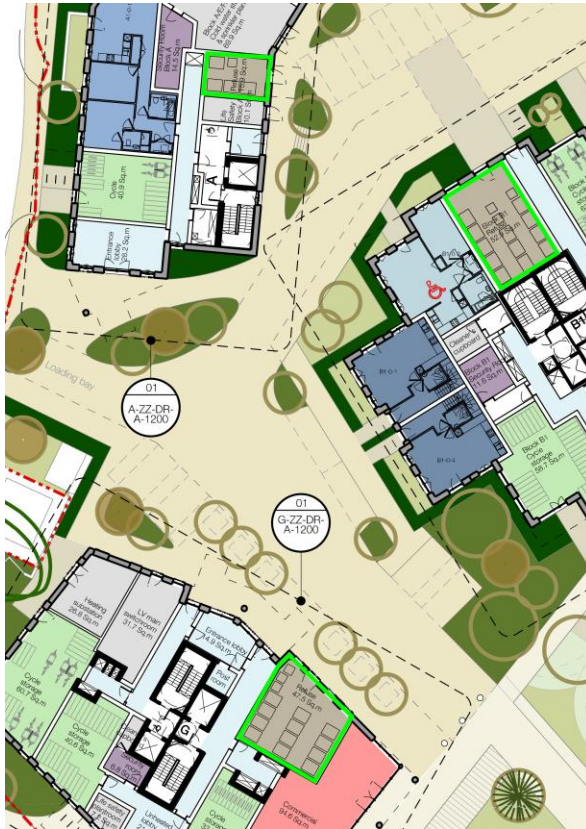
Figure 3-11 Residential Waste Store Configuration – Plots D1/D2/E/F
