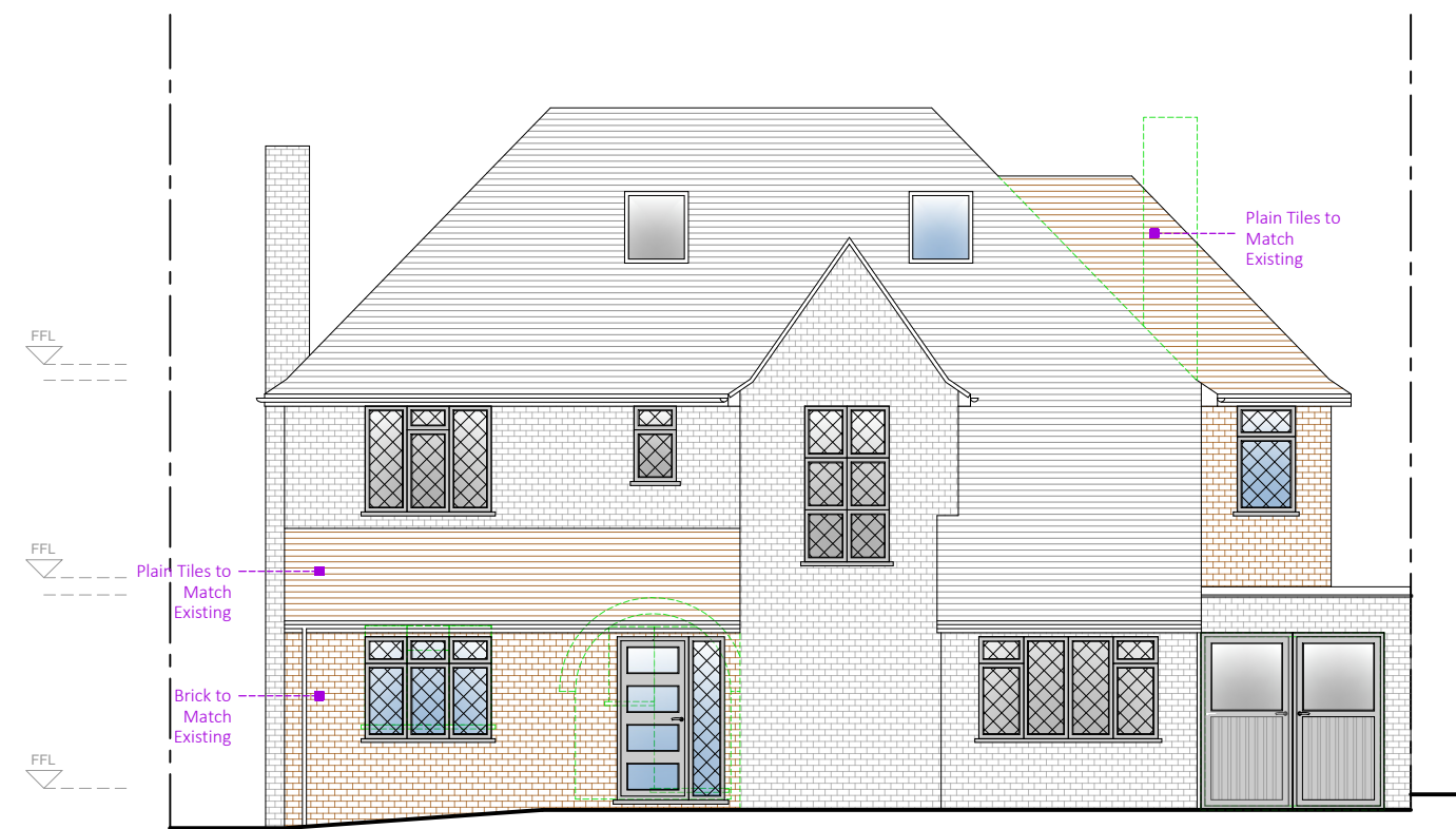
14 Proposed Front Elevation SCALE: 1:100
