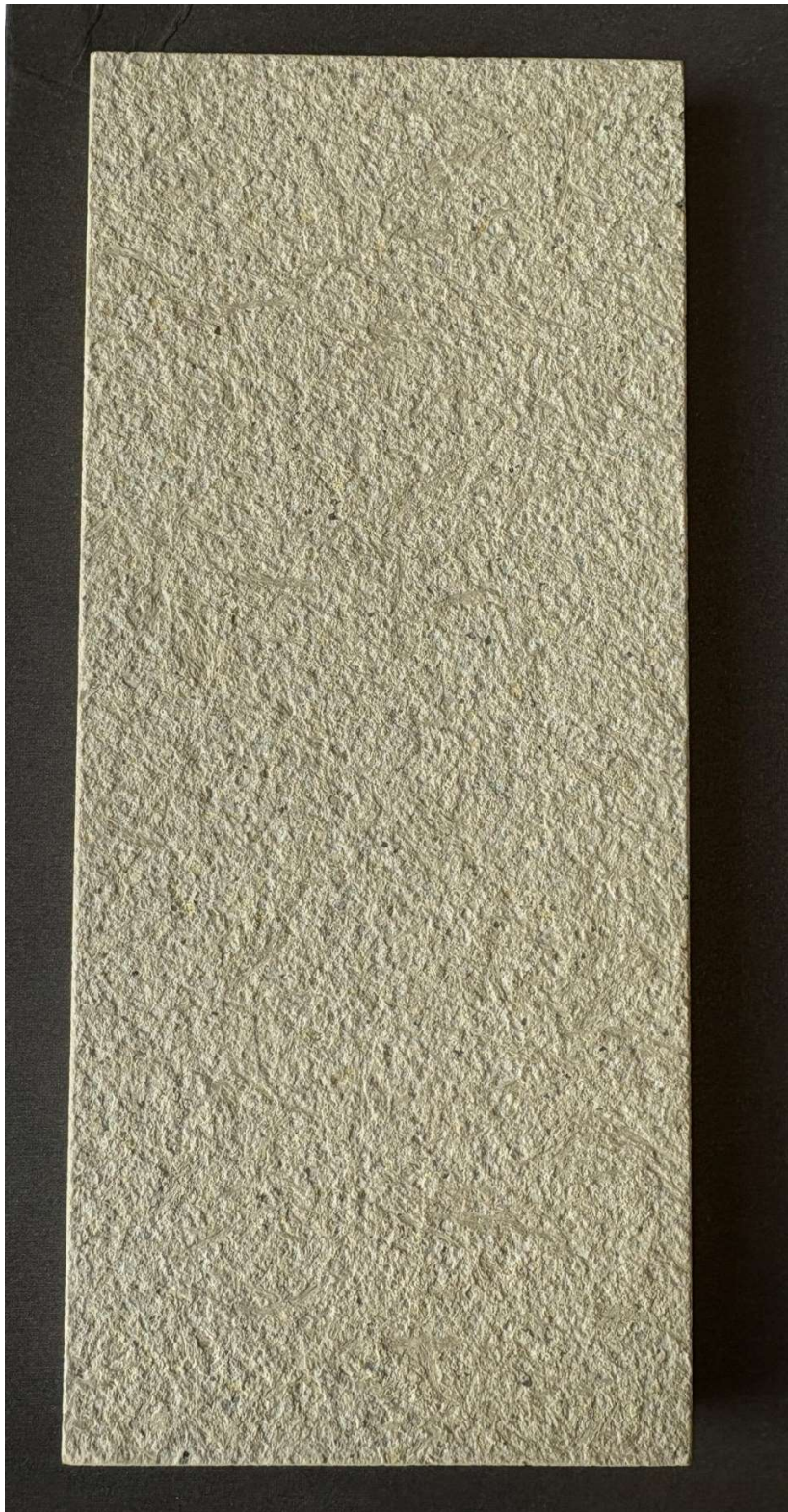
Concrete cladding sample panel Petrarch smooth matt
