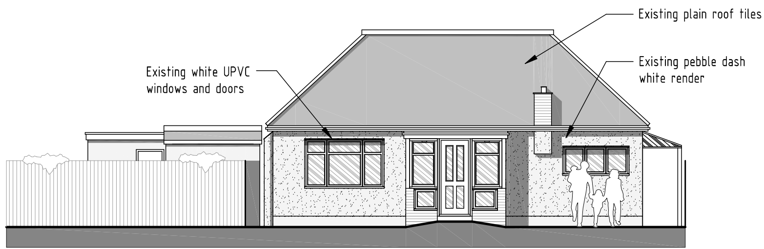
EXISTING REAR ELEVATION
