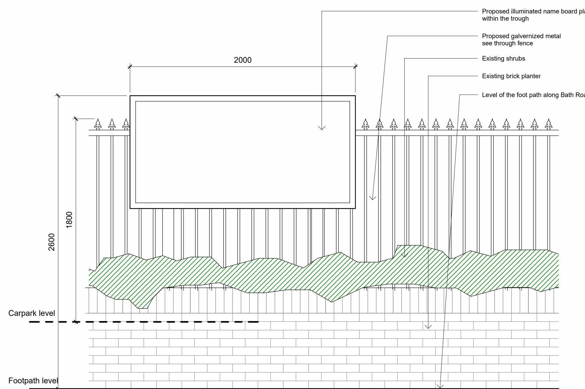
4 Proposed elevation of the name board and metal fence 1:20
