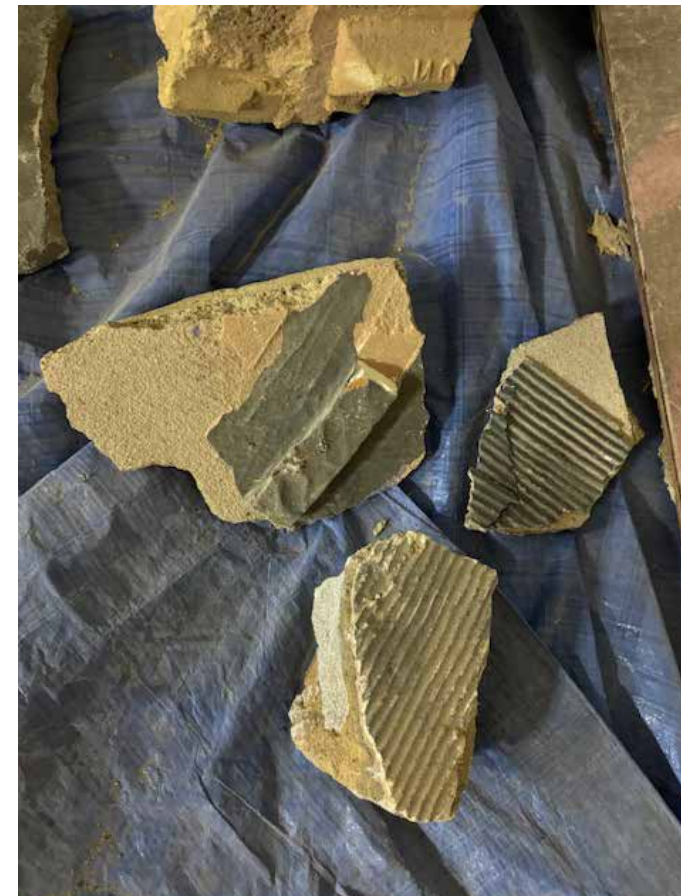
Examples of recovered plaster finishes from the original cinema wall.
