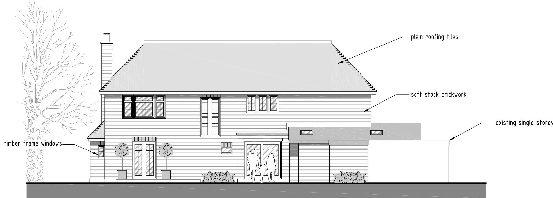
EXISTING REAR ELEVATION - 1:100
