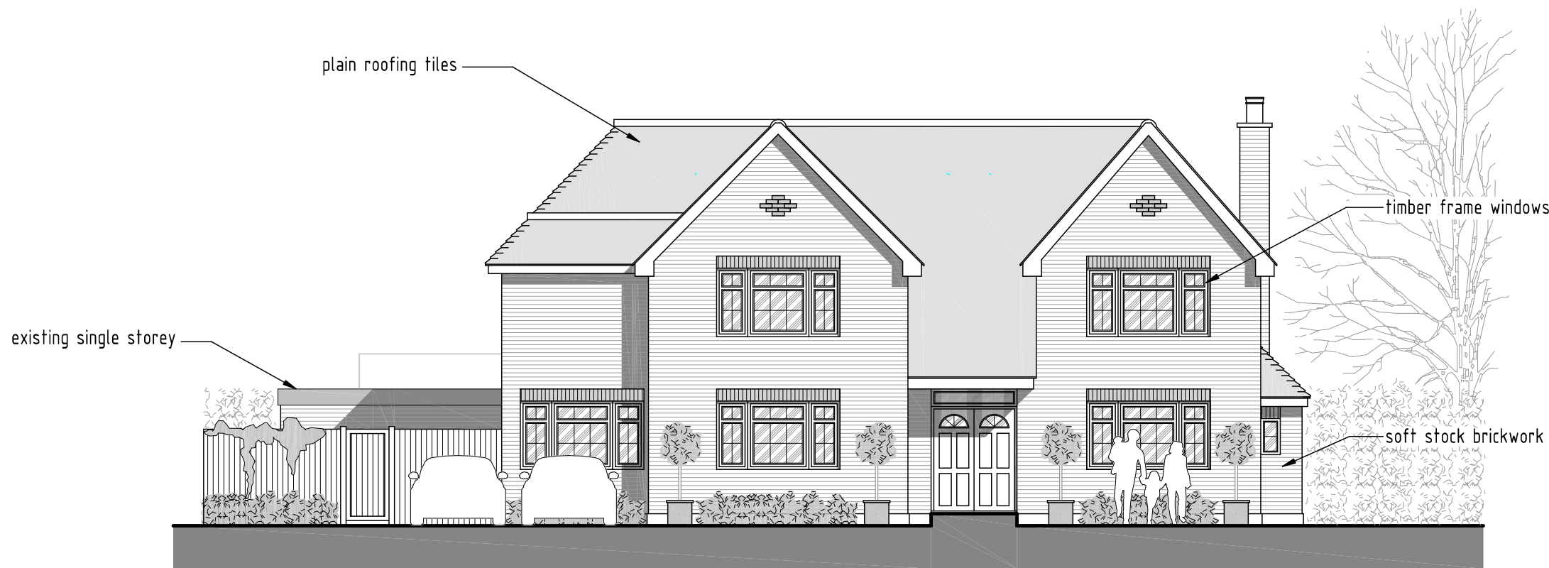
EXISTING FRONT ELEVATION - 1:100
