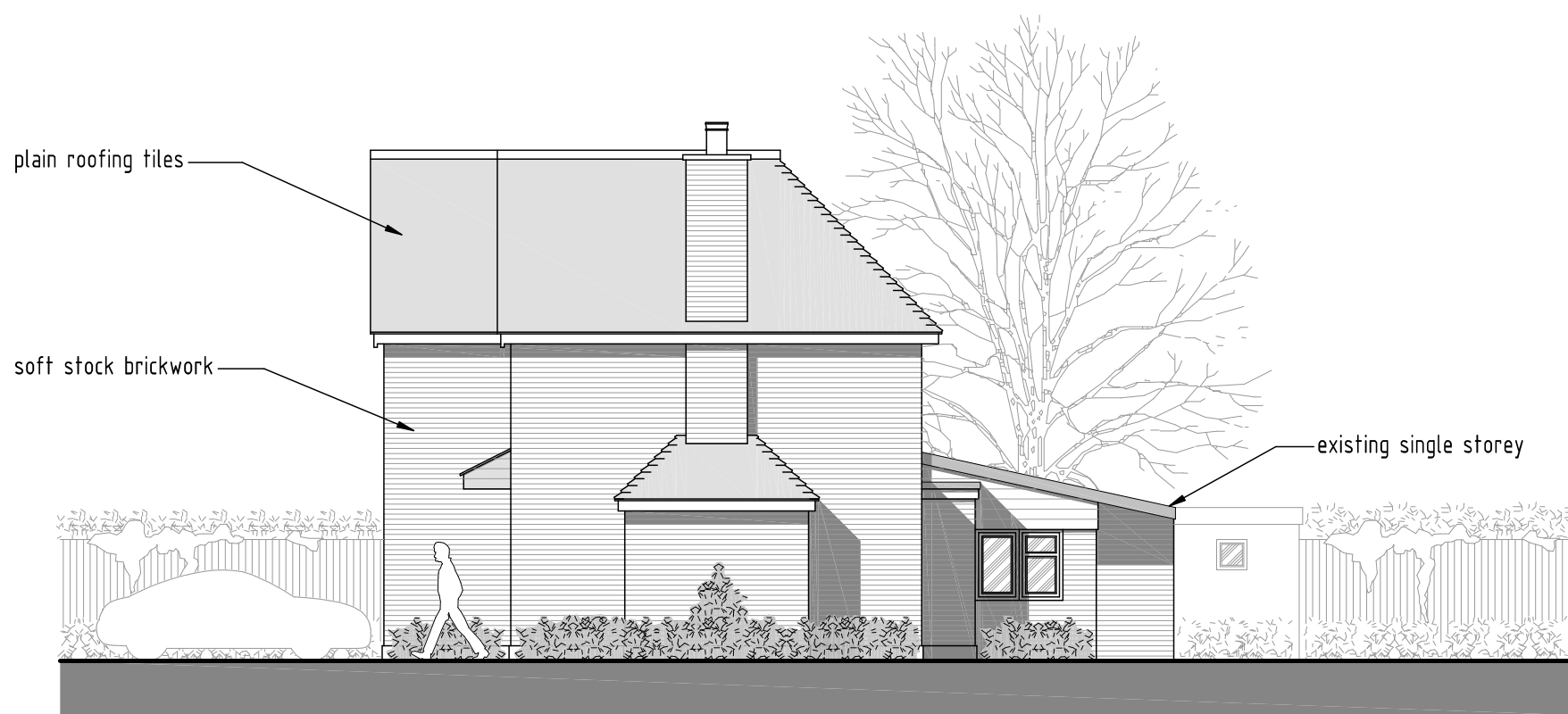
EXISTING SIDE ELEVATION - 1:100
