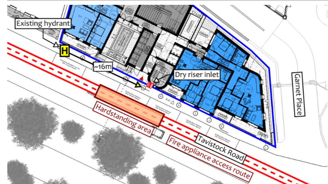
Figure 12 – Firefighting vehicle access and water supplies
