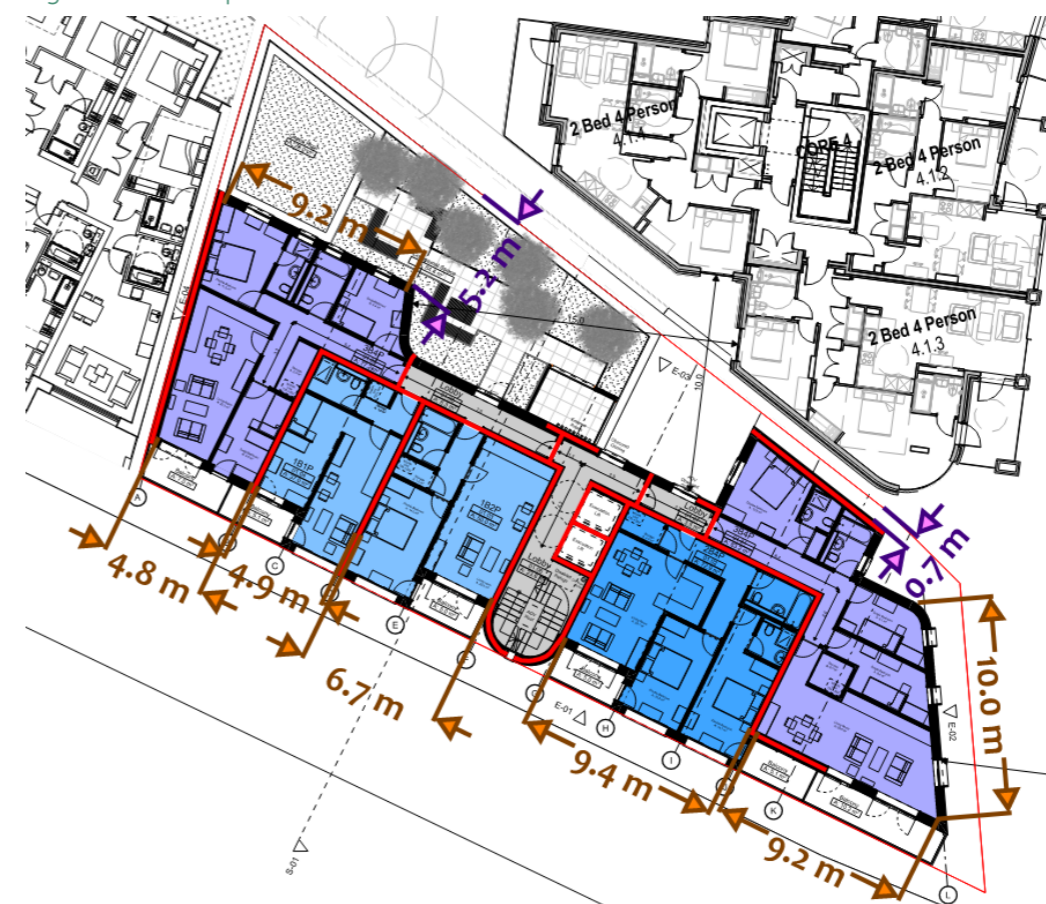
Figure 11 – Compartment dimensions at First Floor
