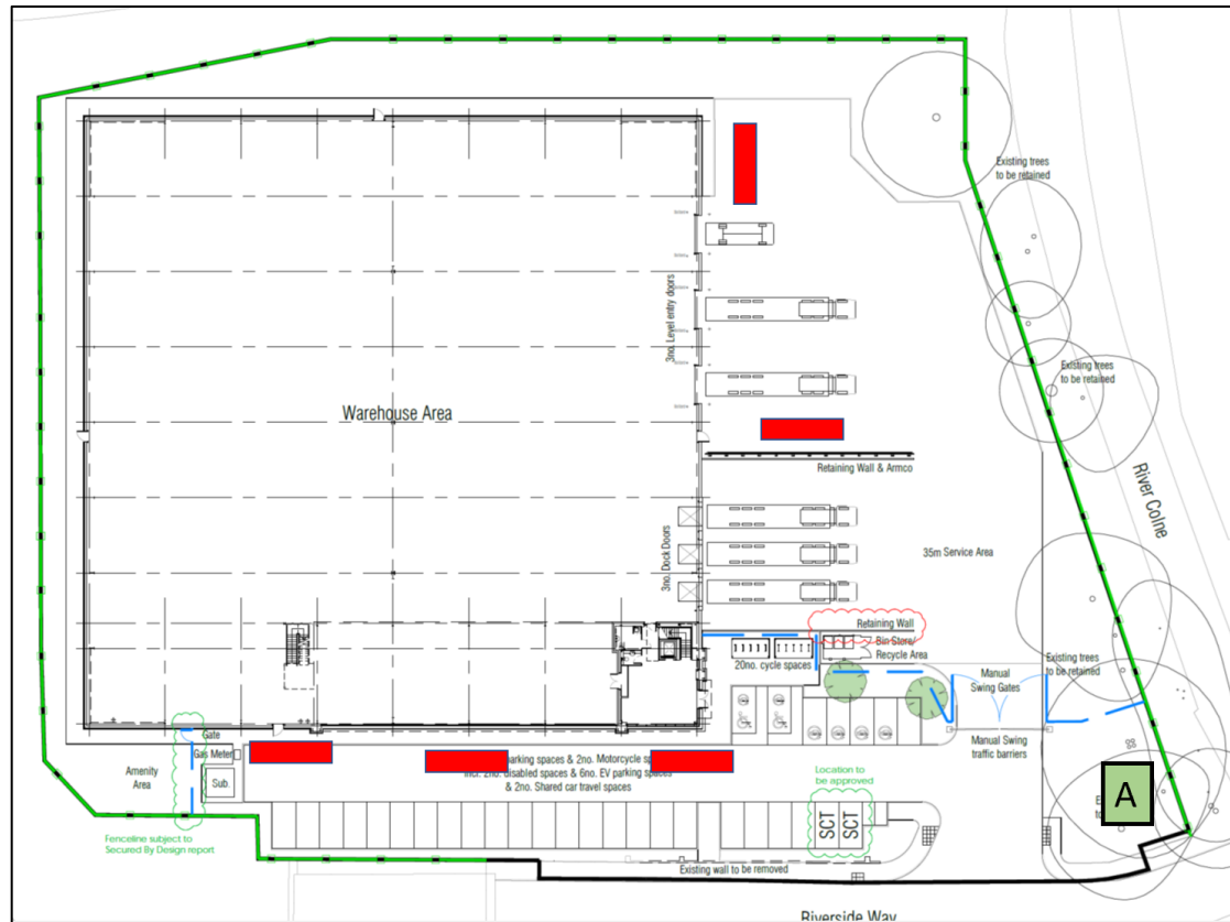
Figure 5 - Site plan showing potential appliance access to the east and south elevations
