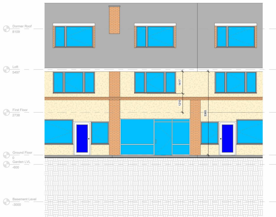
1 Proposed Front Elevation 1 : 50
