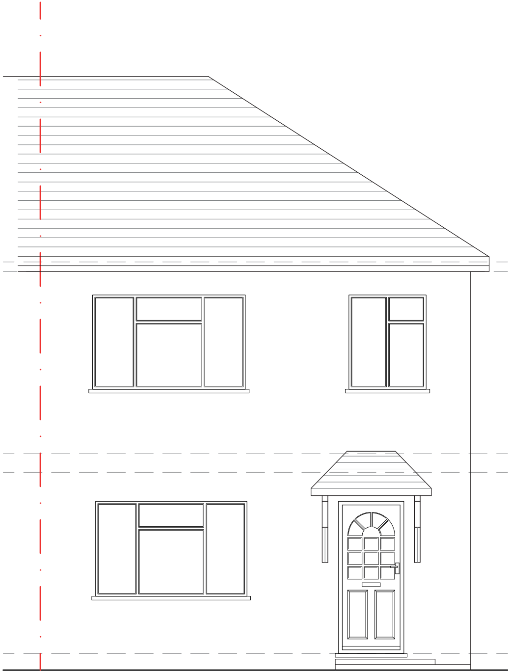
EXISTING FRONT ELEVATION
