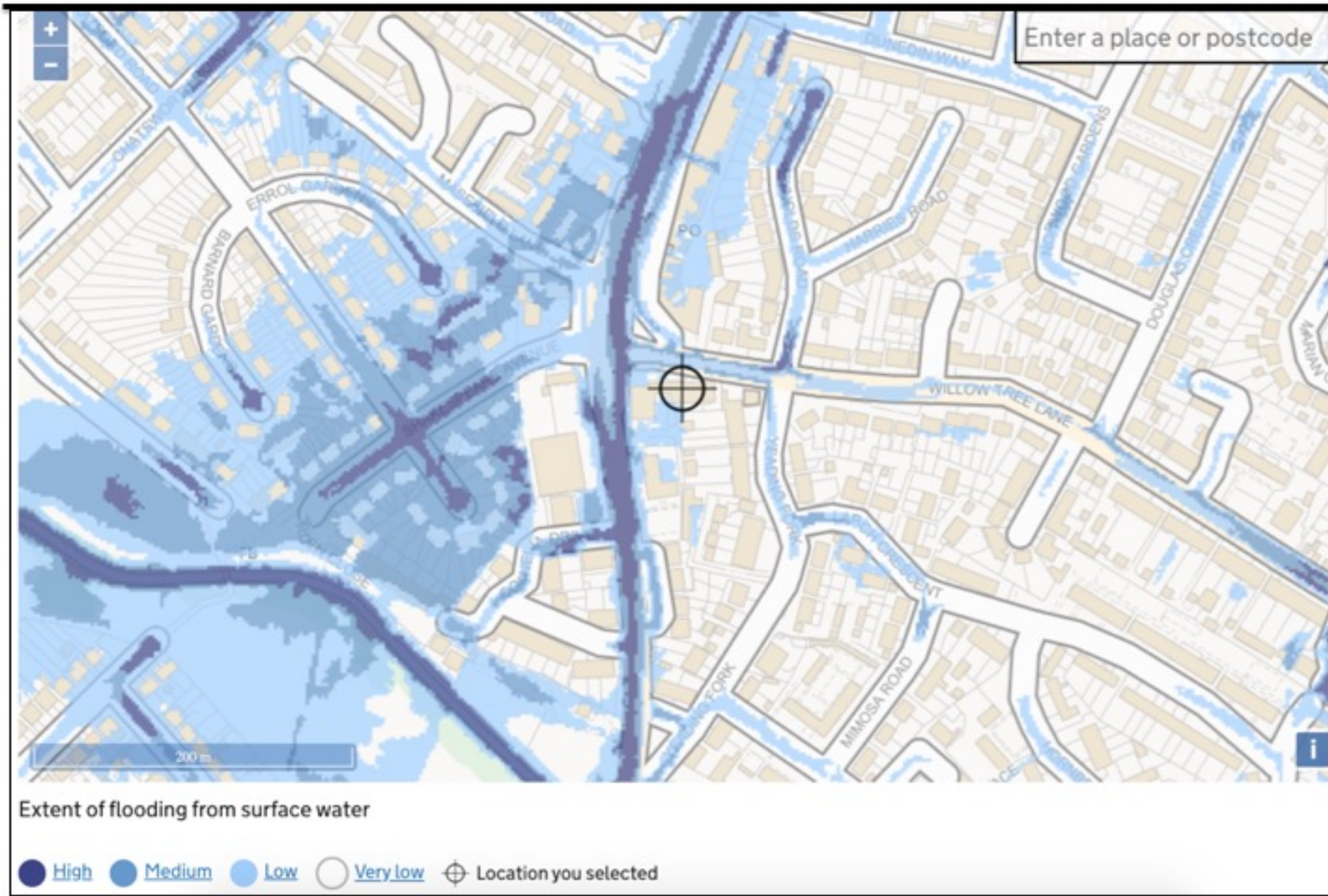
Figure 5 Environment Agency's Surface Water Flood Risk Map
