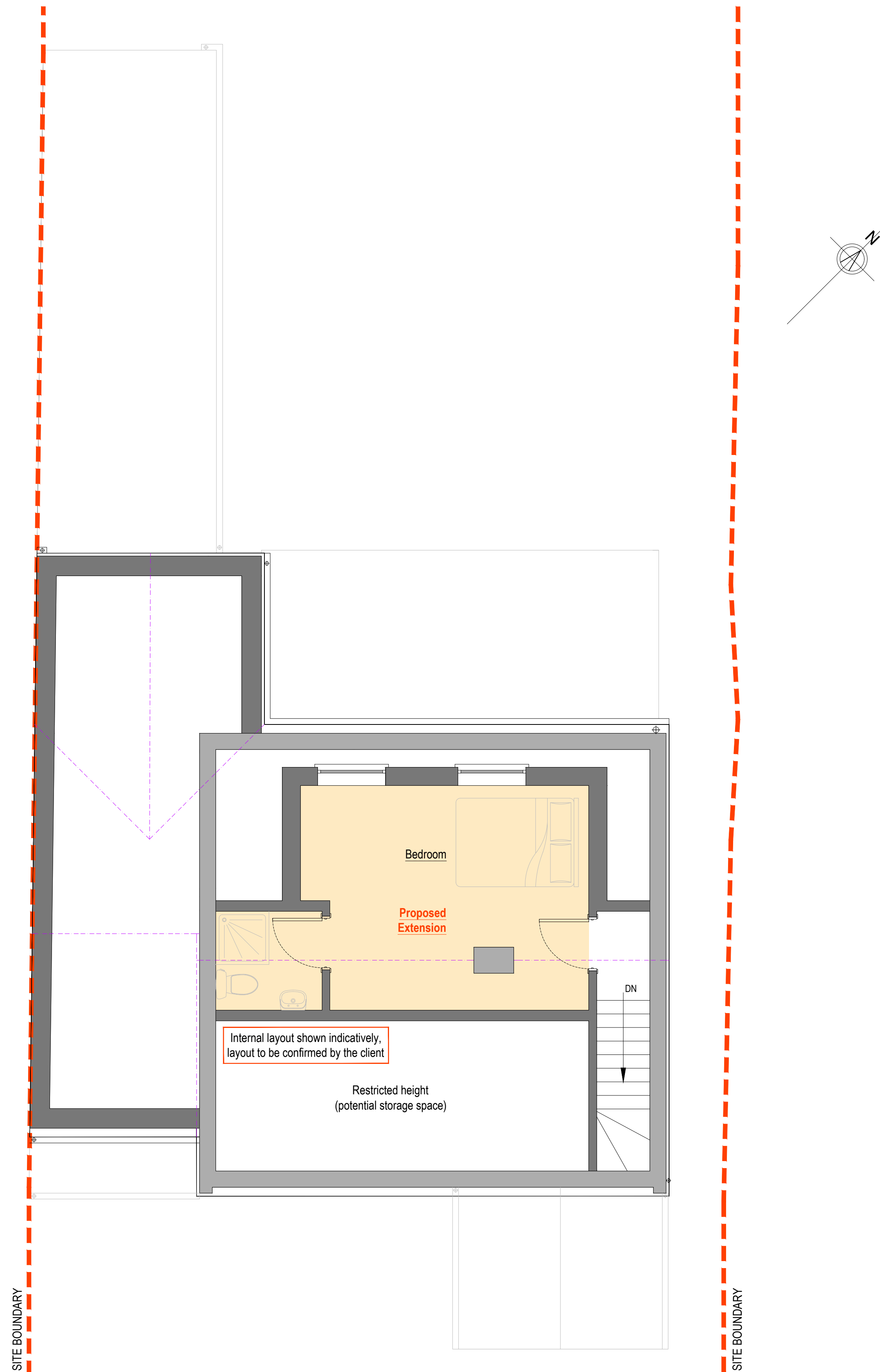
PROPOSED LOFT FLOOR LAYOUT (1:50)
