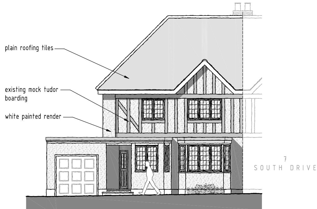
EXISTING FRONT ELEVATION SCALE 1:100
