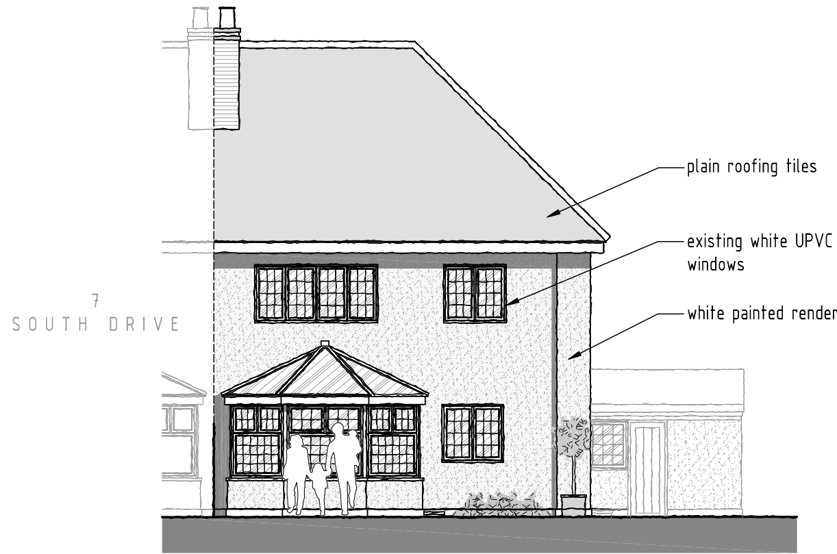
EXISTING REAR ELEVATION SCALE 1:100
