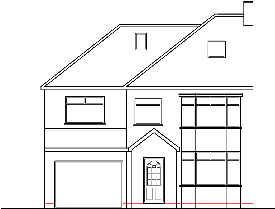
EXISTING FRONT ELEVATION 1:100
