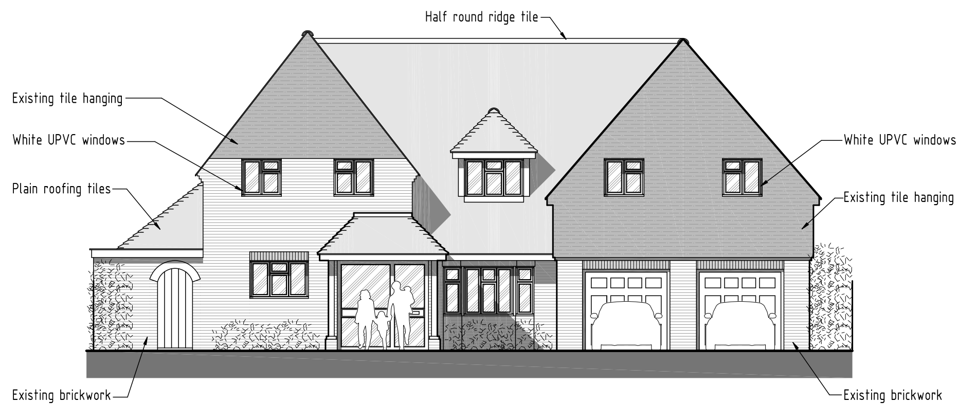
EXISTING FRONT ELEVATION
