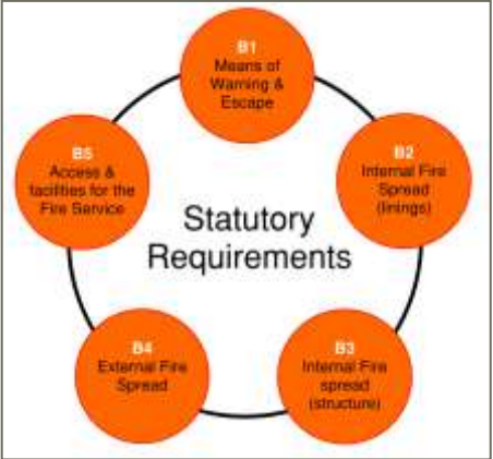
Figure 4: Part B of The Building Regulations
