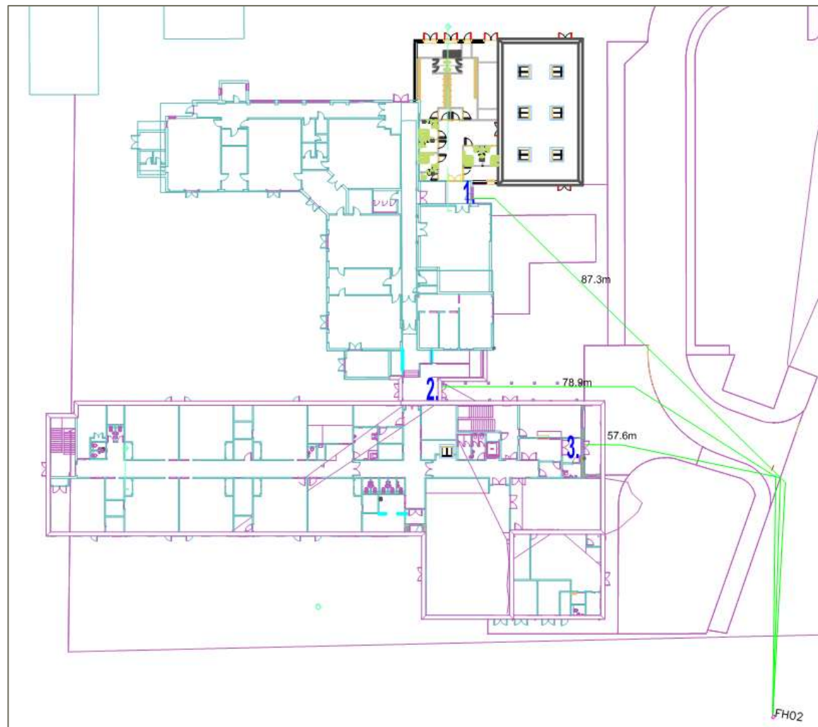
Figure 17: Existing fire hydrant location to the south of the development
