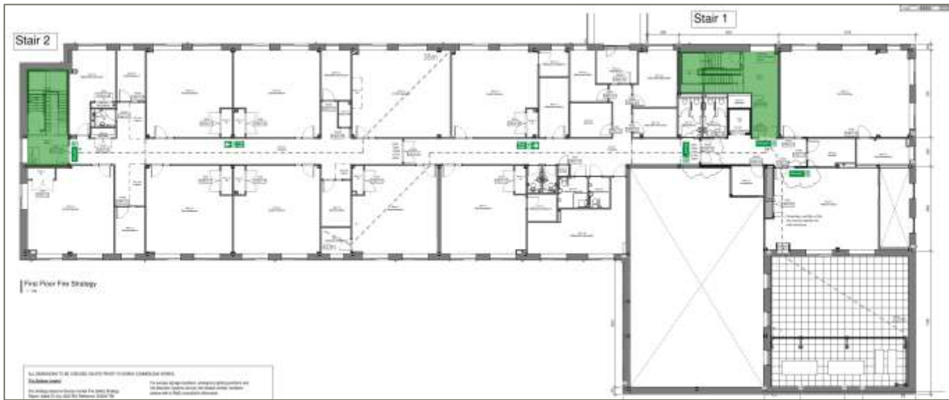
Figure 13: Internal Protected Escape Stairs
