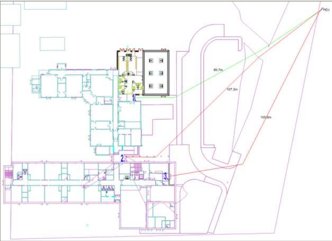
Figure 16: Existing fire hydrant location to the north of the development
