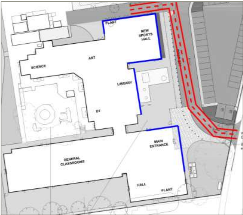
Figure 15: Fire vehicle perimeter access
