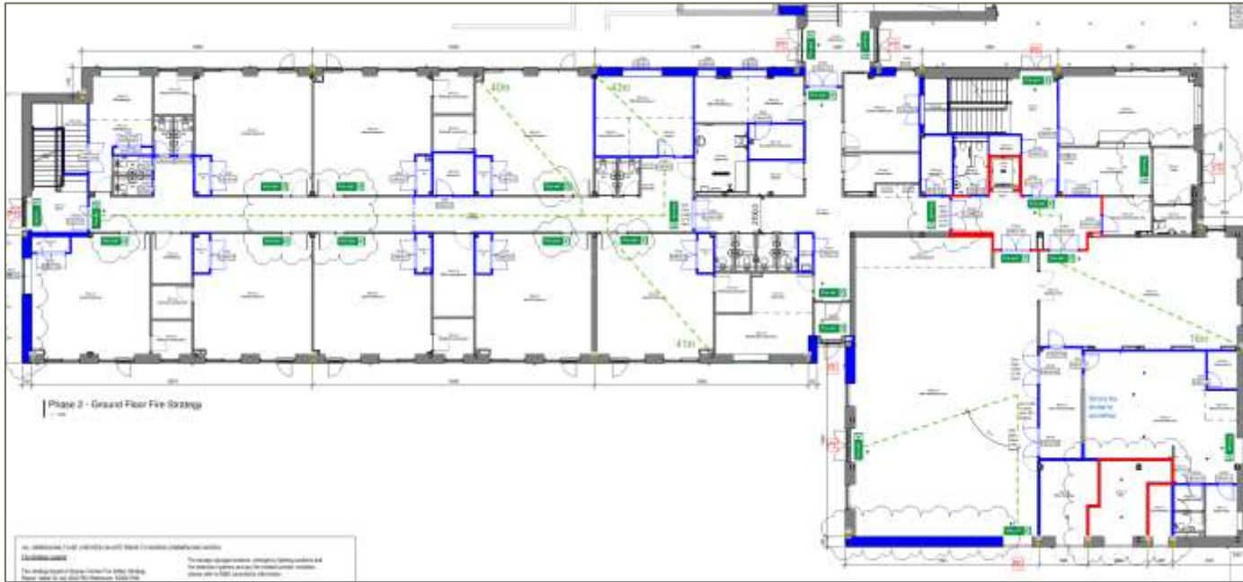
Figure 10: New Build Ground Floor – Escape Doors
