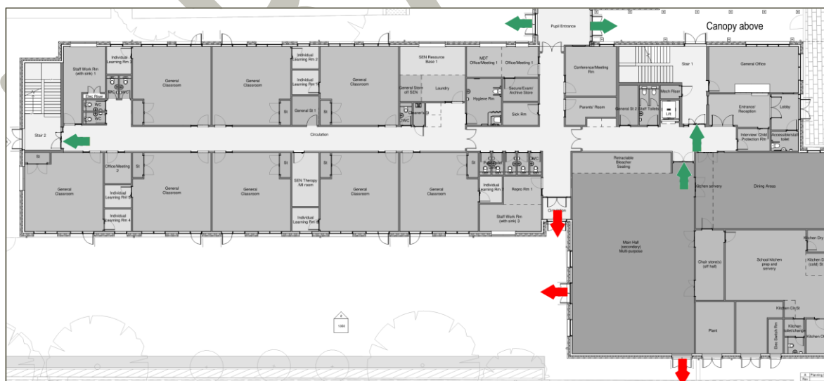
Figure 8: New Build Ground Floor – Escape Doors
