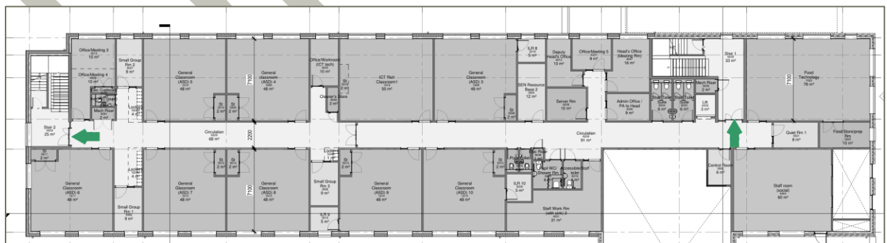
Figure 10: First Floor – Escape Doors
