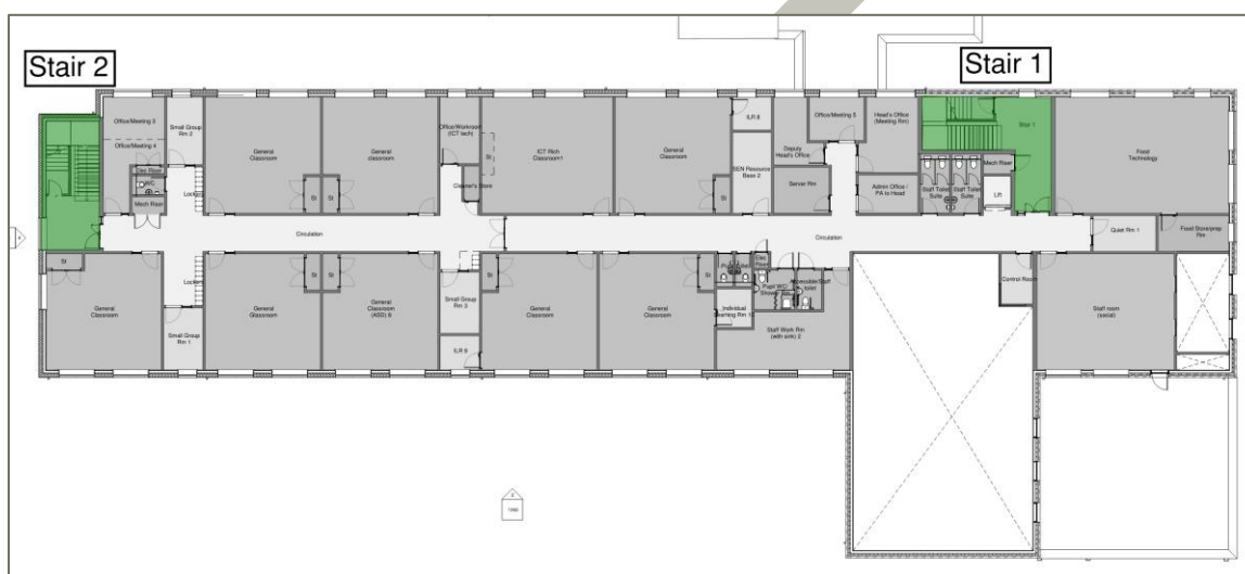
Figure 11: Internal Protected Escape Stairs
