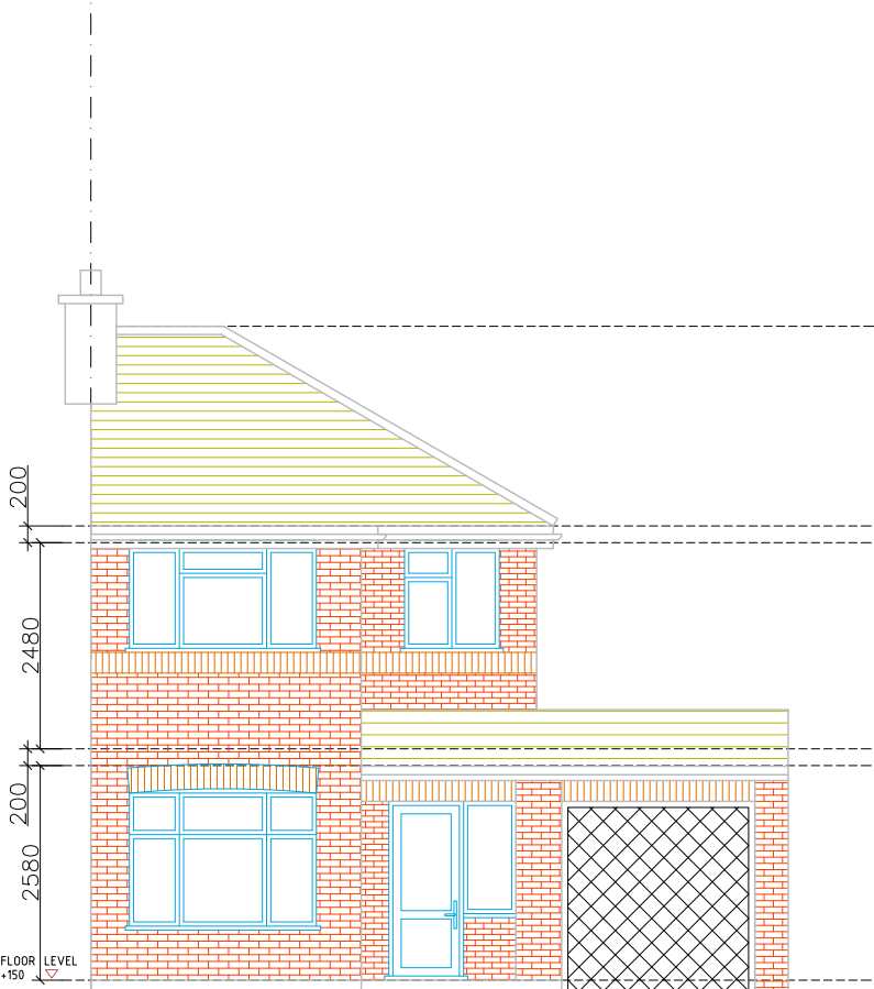
EXISTING FRONT ELEVATION
