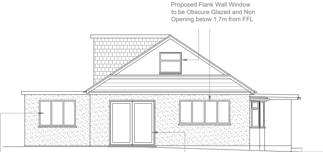
Proposed Side Elevation Scale 1:100
