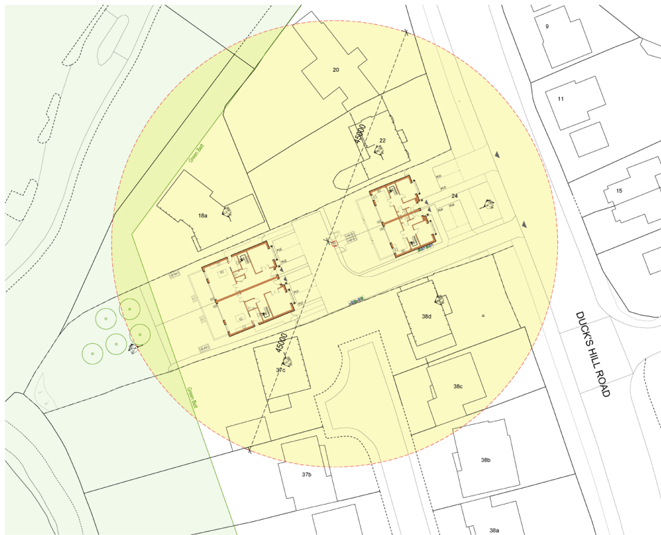
Figure 22 – Proposed fire safety site plan based on hydrant coverage
