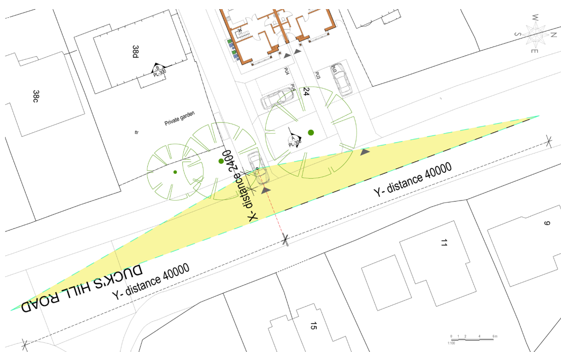
Figure 19 – Proposed Site Plan Traffic Splay Diagram.
