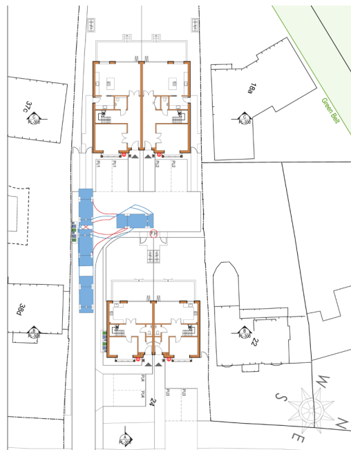
Figure 21 – Proposed traffic swept path diagram for ambulance '3-point turn'
