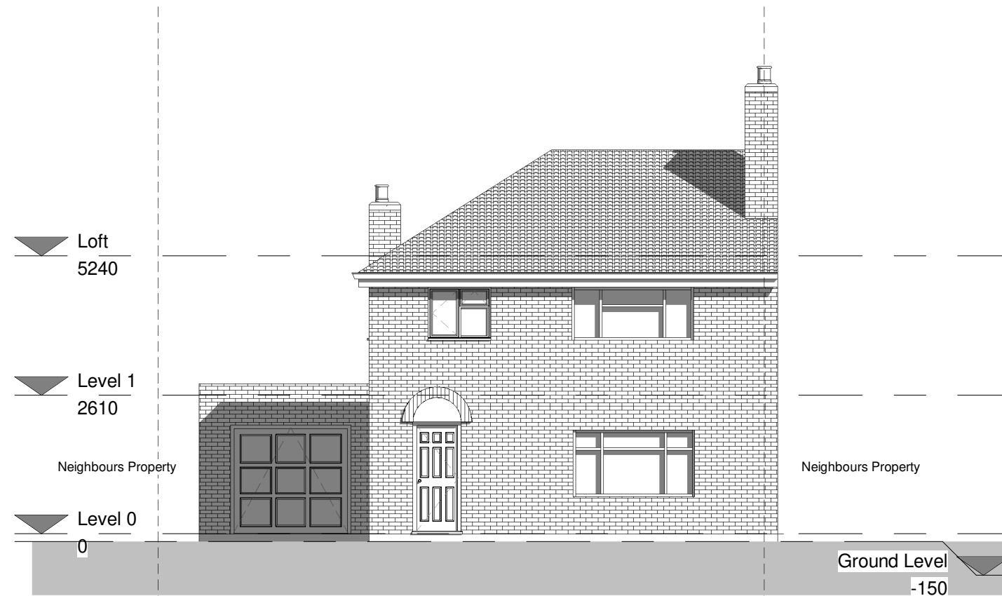
1 Front elevation - Existing 1 : 100
