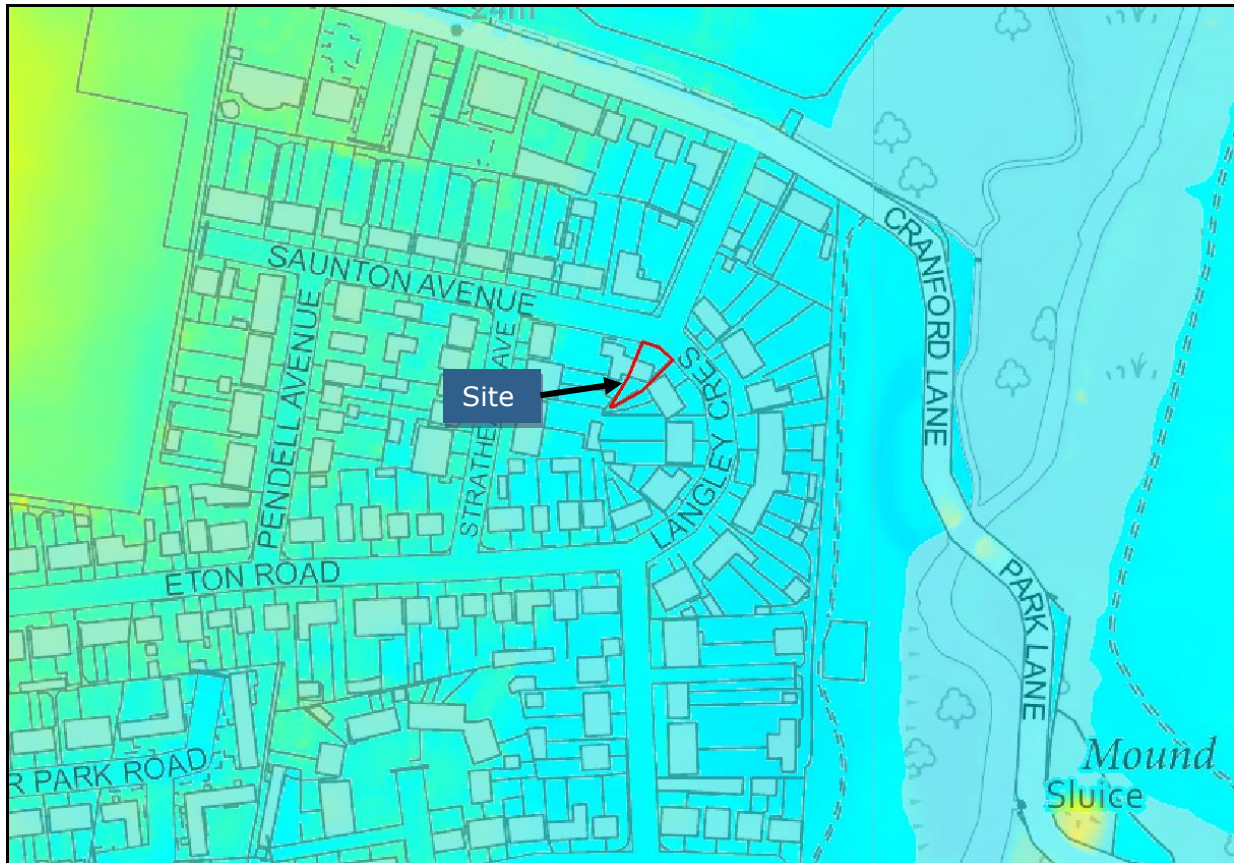
Figure 2: LIDAR survey data where higher ground is denoted as red, orange and yellow colours and lower areas denoted by blue and green colours
