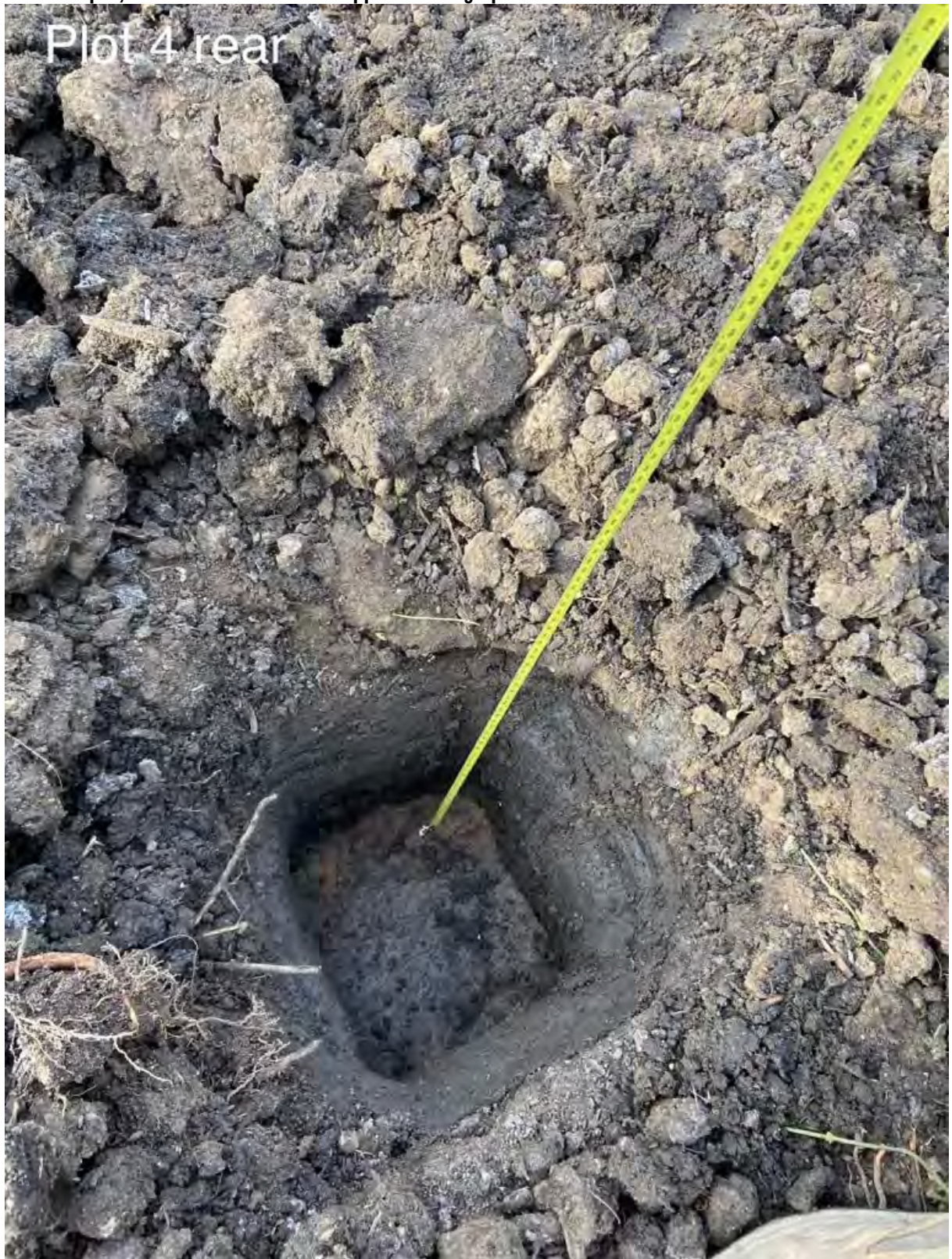
Photograph 15: Verification pit advanced within rear garden of Plot 4.
