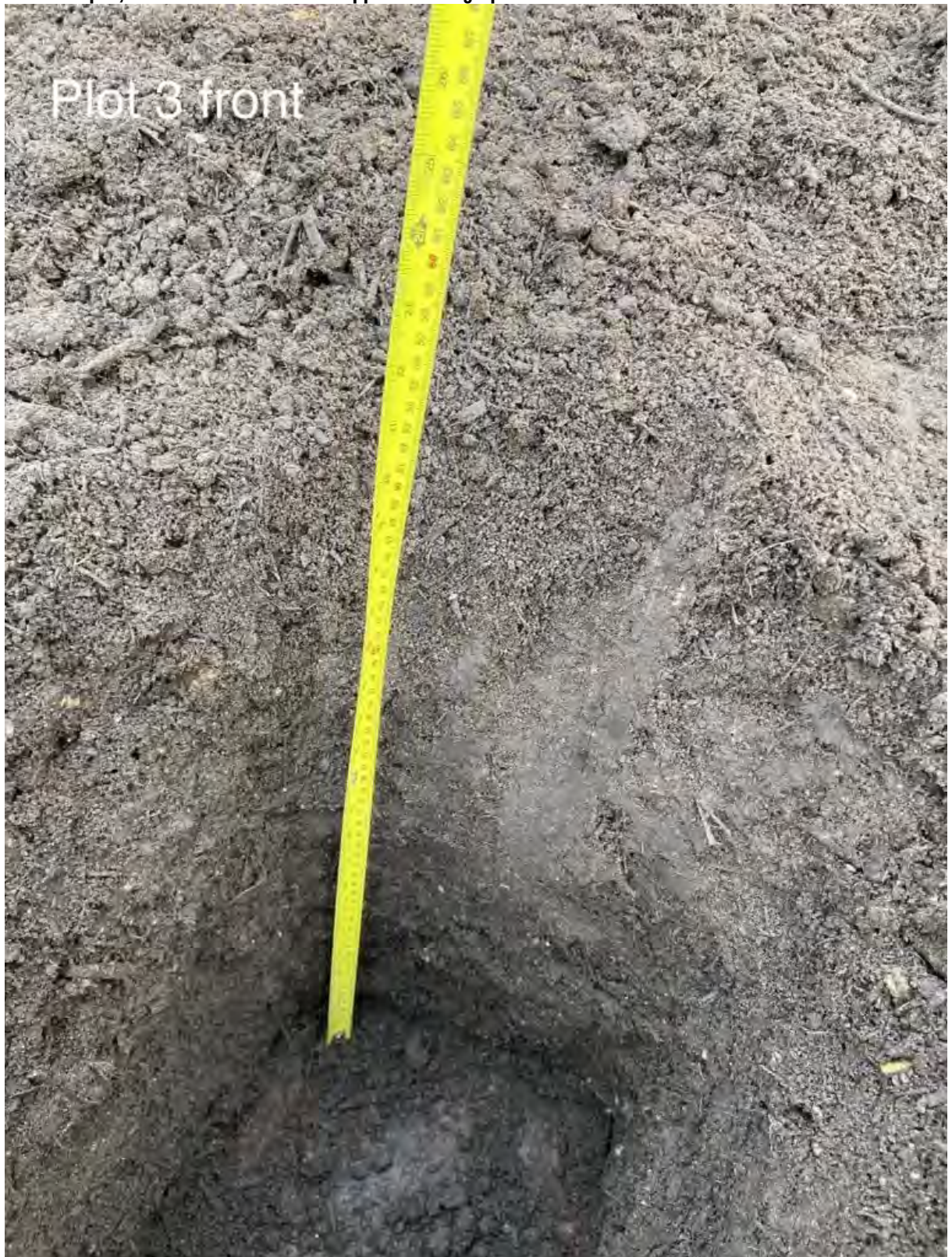
Photograph 10: Verification pit advanced within front garden of Plot 3.
